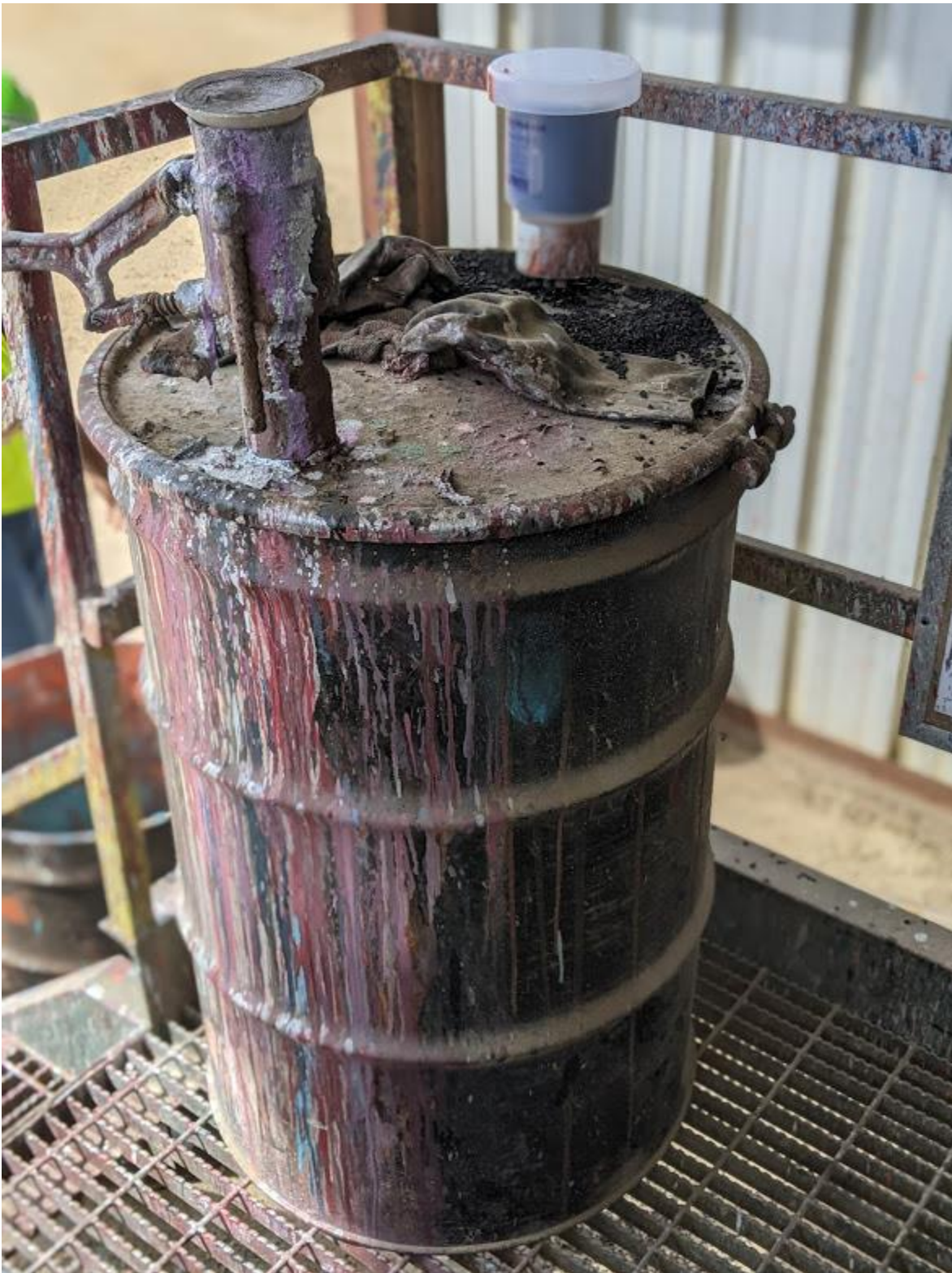
Photograph 1 of 3: SAA Container for hazardous waste from punctured aerosols
