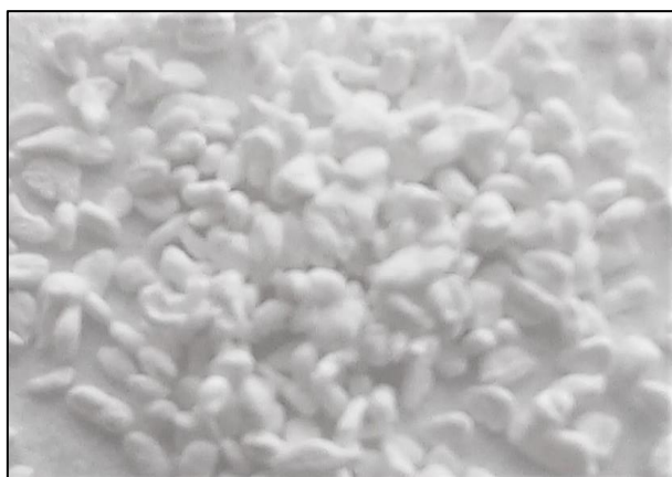
Figure 3. Recycled PVDF Solef® PVDF from “end of life” hollow fibers
