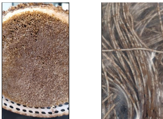
Figure 1. “End of life” PVDF hollow fibers
