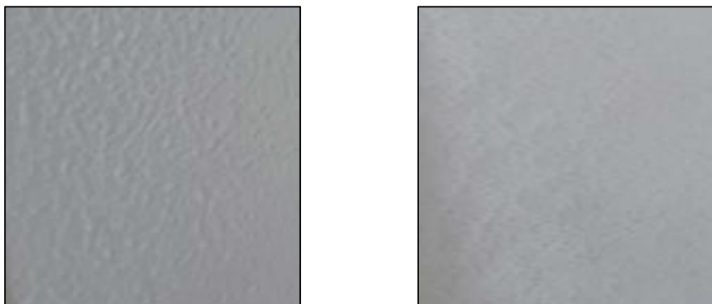
Figure 4. Membranes cast from Virgin Solef® PVDF (left) and recycled Solef® PVDF (right)
