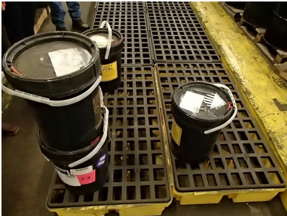
Photo 4: A closer view of the 4 PCB 5-gallon containers in Photo 3. Two containers had PCB M L marks on the outside of the containers and 2 containers did not. None of the PCB containers had a removed from service date.
