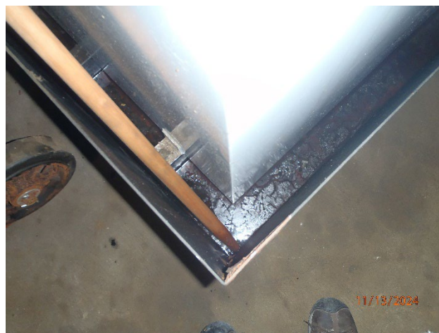
Picture 16 – Spinning Maintenance Used Oil need cleanout
