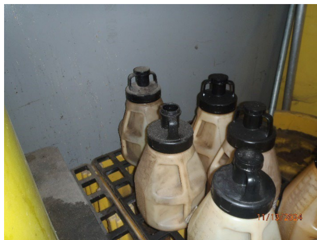
Picture 4 – CARB Used Oil containers – one not closed
