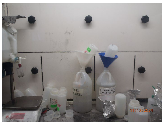
Picture 41 – CARB Lab 1 fume hood SAA open containers
