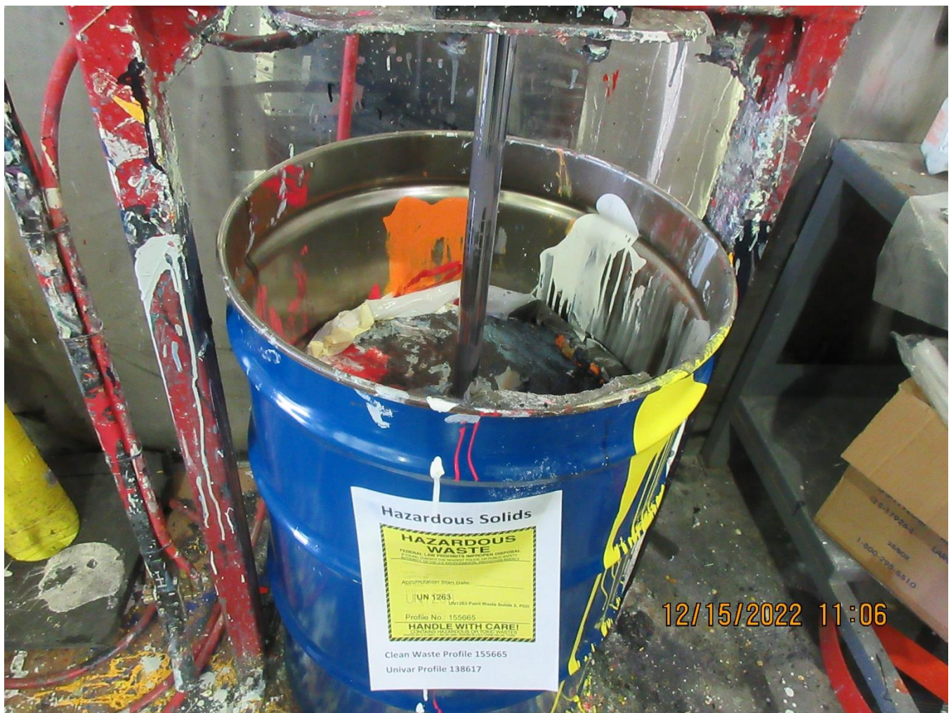
Photo 25 – Top of drum of hazardous waste solids and crushing device along the southern wall of the Cleaning Area.
