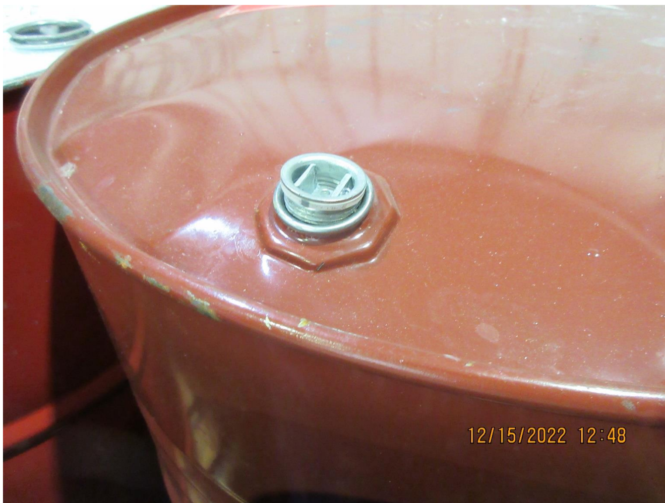
Photo 47 - Bung missing on bulging drum in BLD drum position on pallet in T2 pallet position
