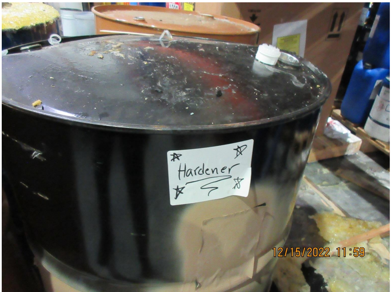
Photo 34 – Drum of Hardener with bulging lid in BRD drum position on pallet B4.
