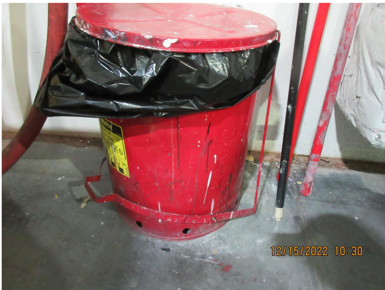
Photo 4 – One of two 12-gallon containers of hazardous waste near a workstation in Scratch-On Production Area
