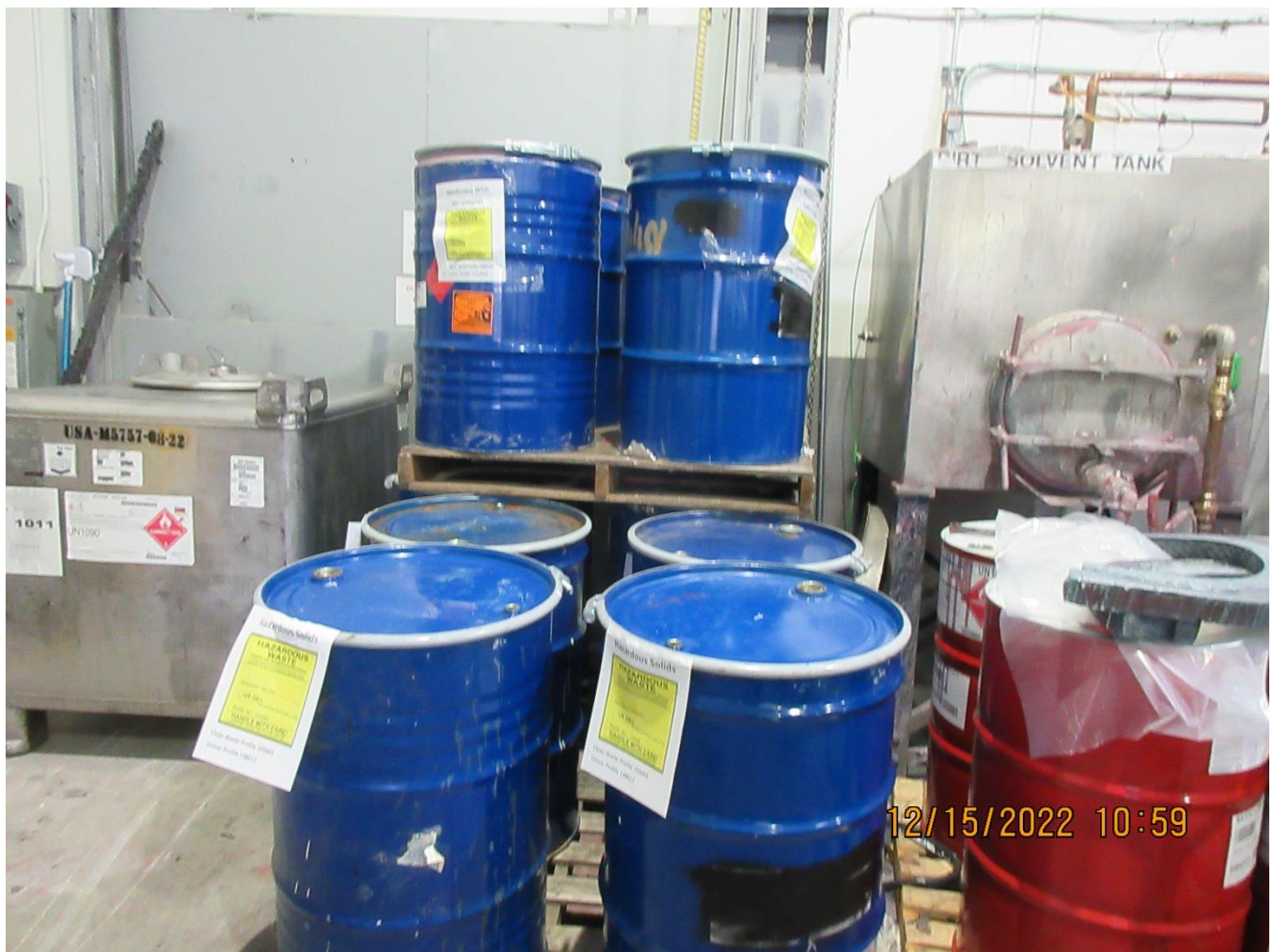
Photo 17 – Twelve 55-gallon drums (blue) of hazardous waste spent solvents observed on pallets on western interior wall.
