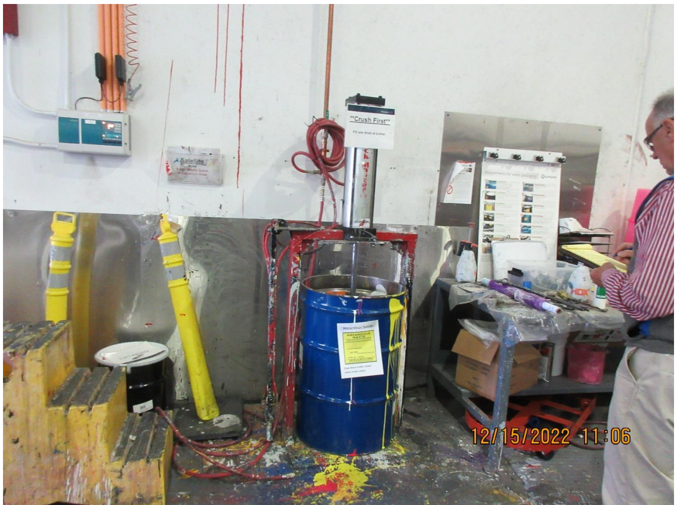
Photo 23 – Drum of hazardous waste solids and crushing device along the southern wall of the Cleaning Area.
