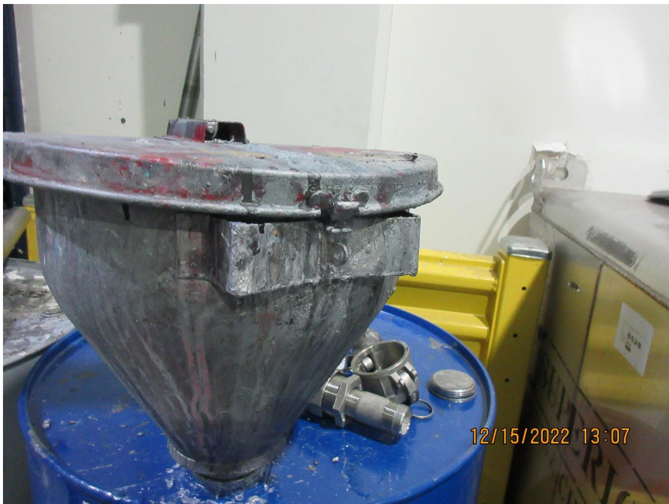
Photo 54 – Funnel with no latch on 55-gallon drum in Metallic Area
