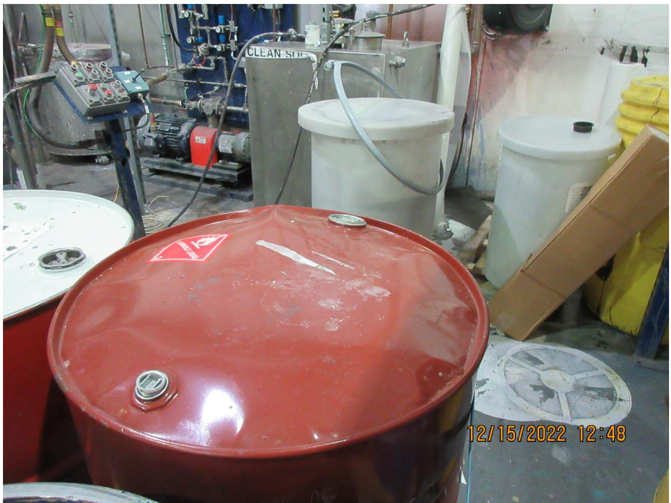
Photo 48 - Bung missing on bulging drum in BLD drum position on pallet in T2 pallet position
