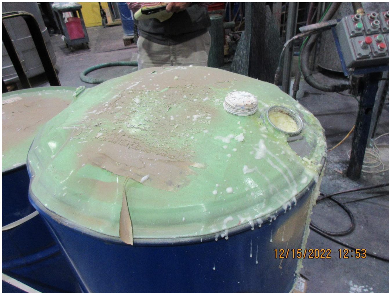
Photo 50 - Bung missing on bulging drum in BRD drum position on pallet in T1 pallet position
