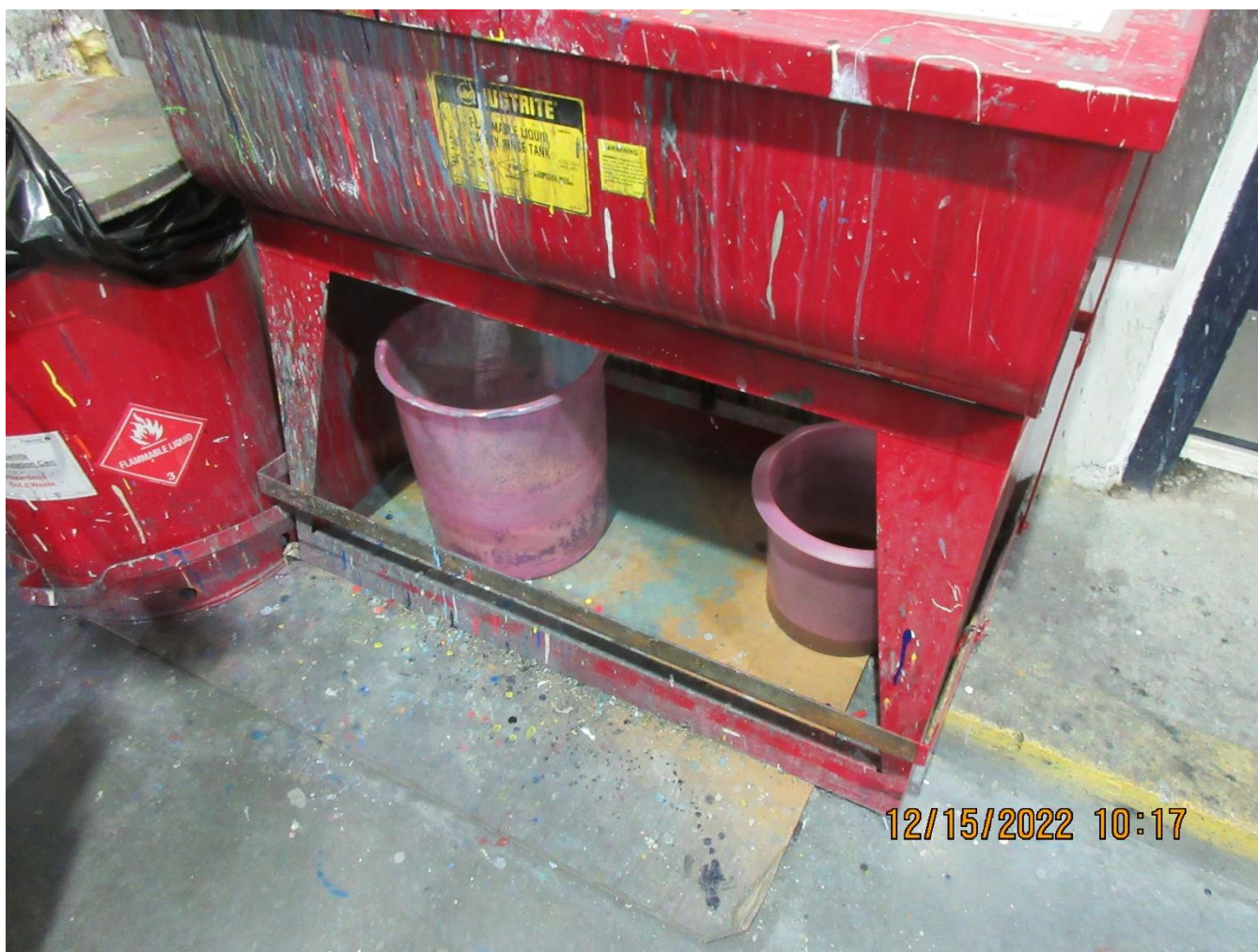
Photo 2 – Containers of in-use solvents beneath solvent cleaning machine in the Tinting Area
