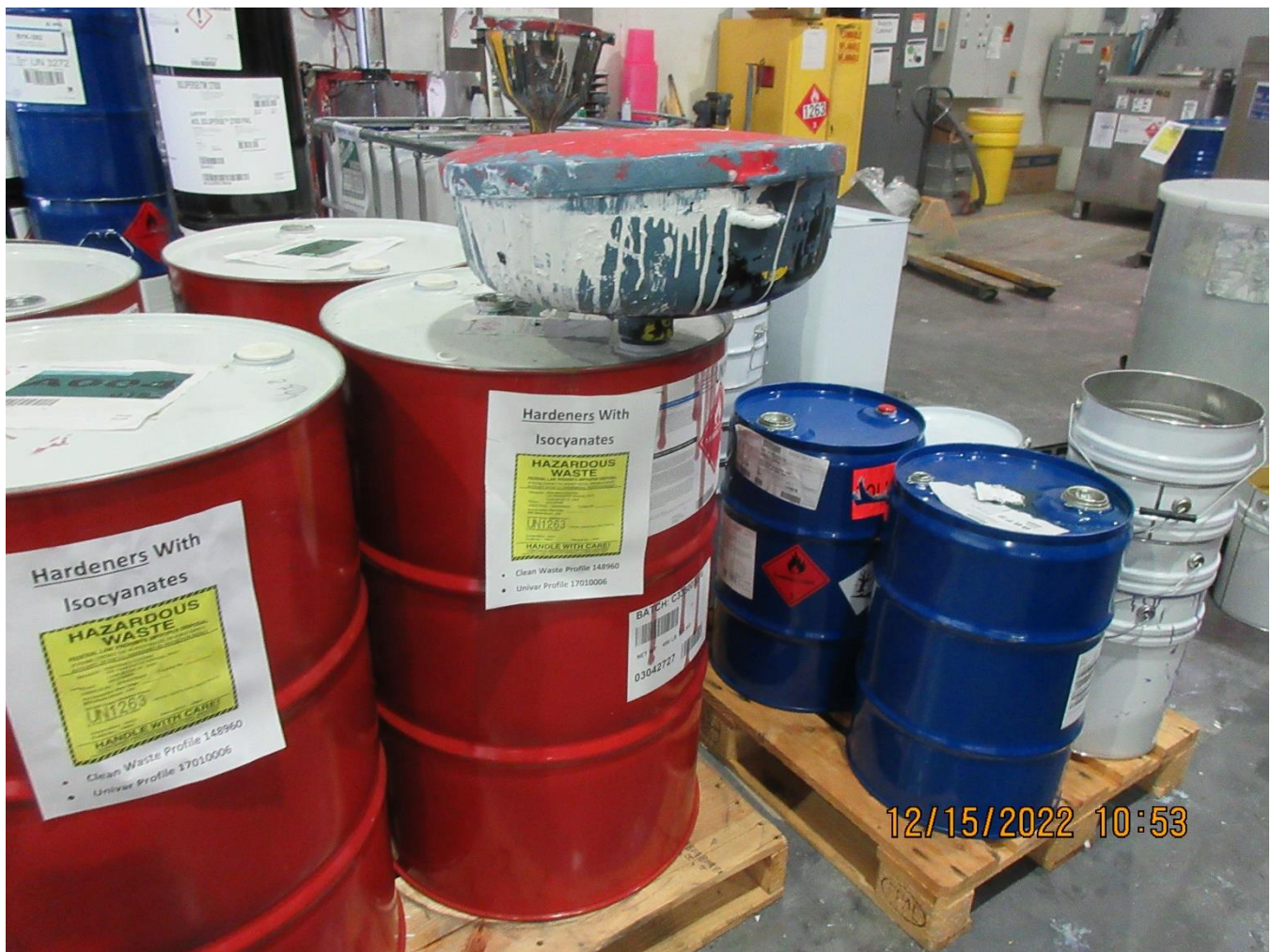
Photo 16 – Pallet with two red 55-gallon drum of hazardous waste hardeners with isocyanates w/o accumulation start dates.
