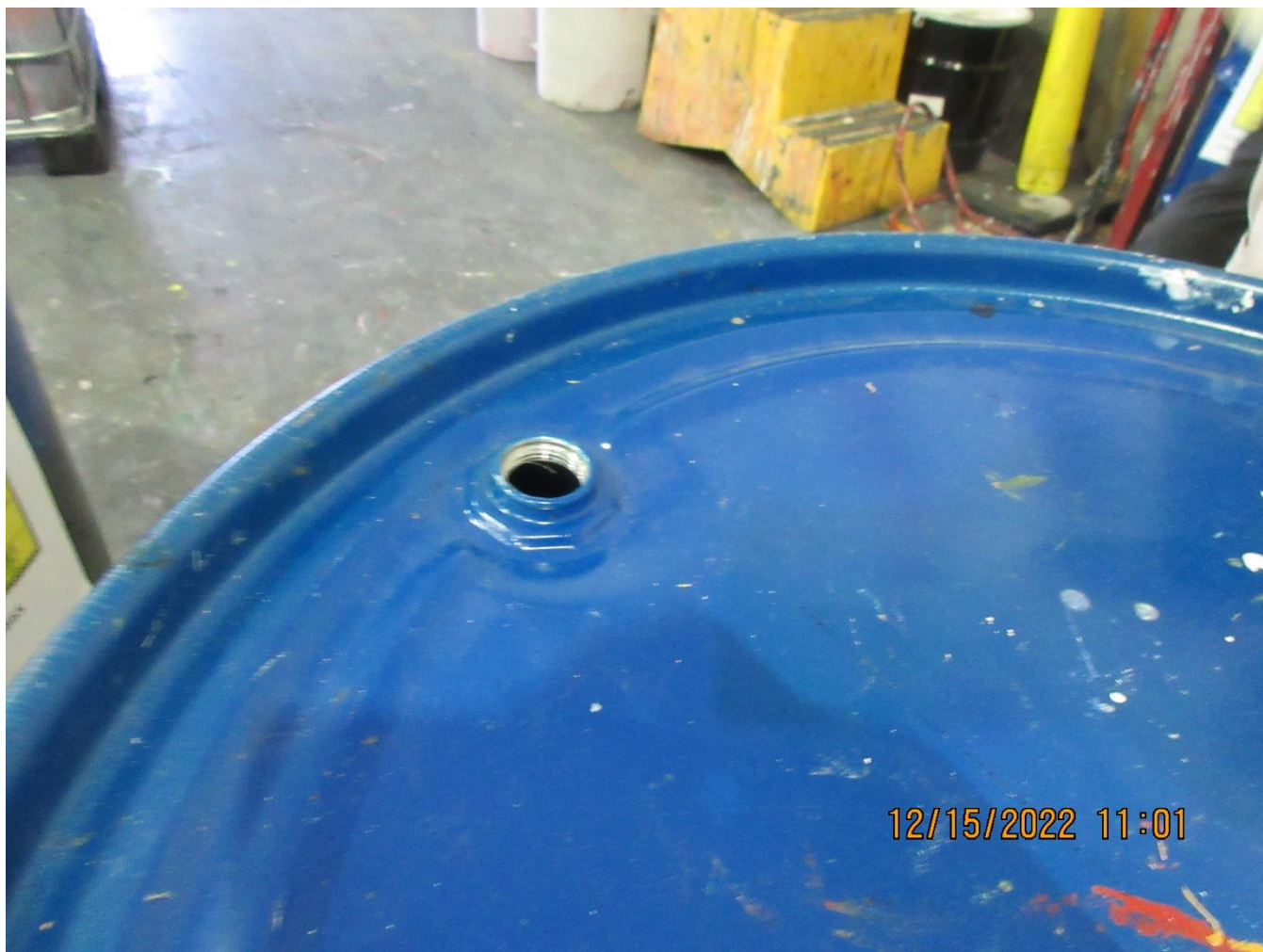
Photo 19 – Open drum (missing bung) of hazardous waste spent solvents on right side of pallet as shown in Photo 18.
