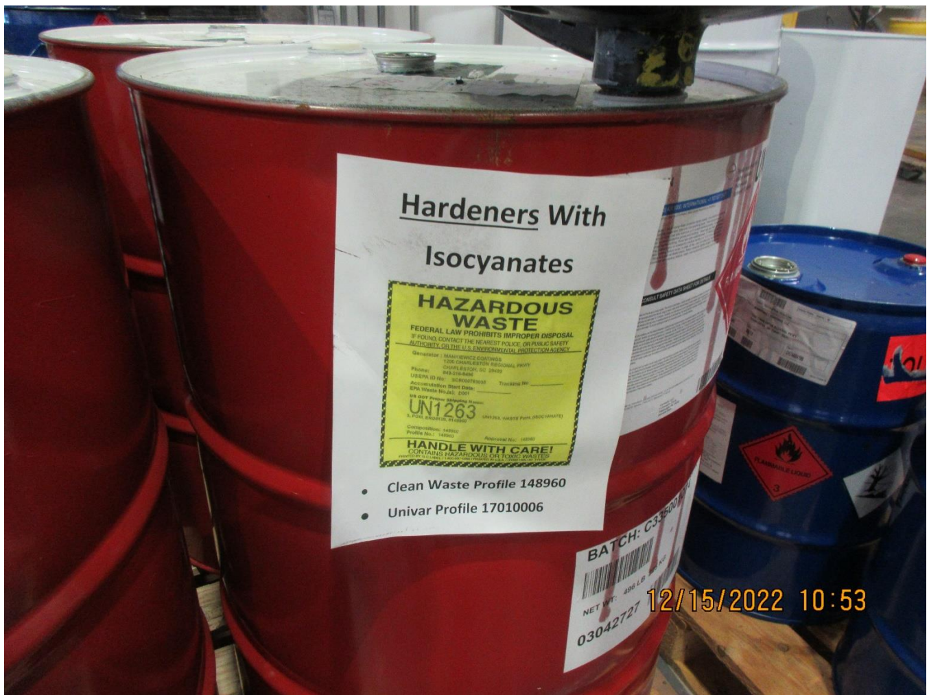
Photo 15 –Label on 55-gallon drum of hazardous waste hardeners with isocyanates w/o accumulation start dates.
