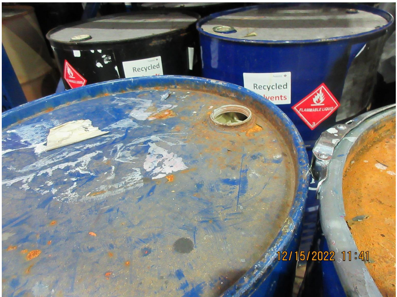
Photo 32 – Bung missing on RLD drum on Pallet FB5
