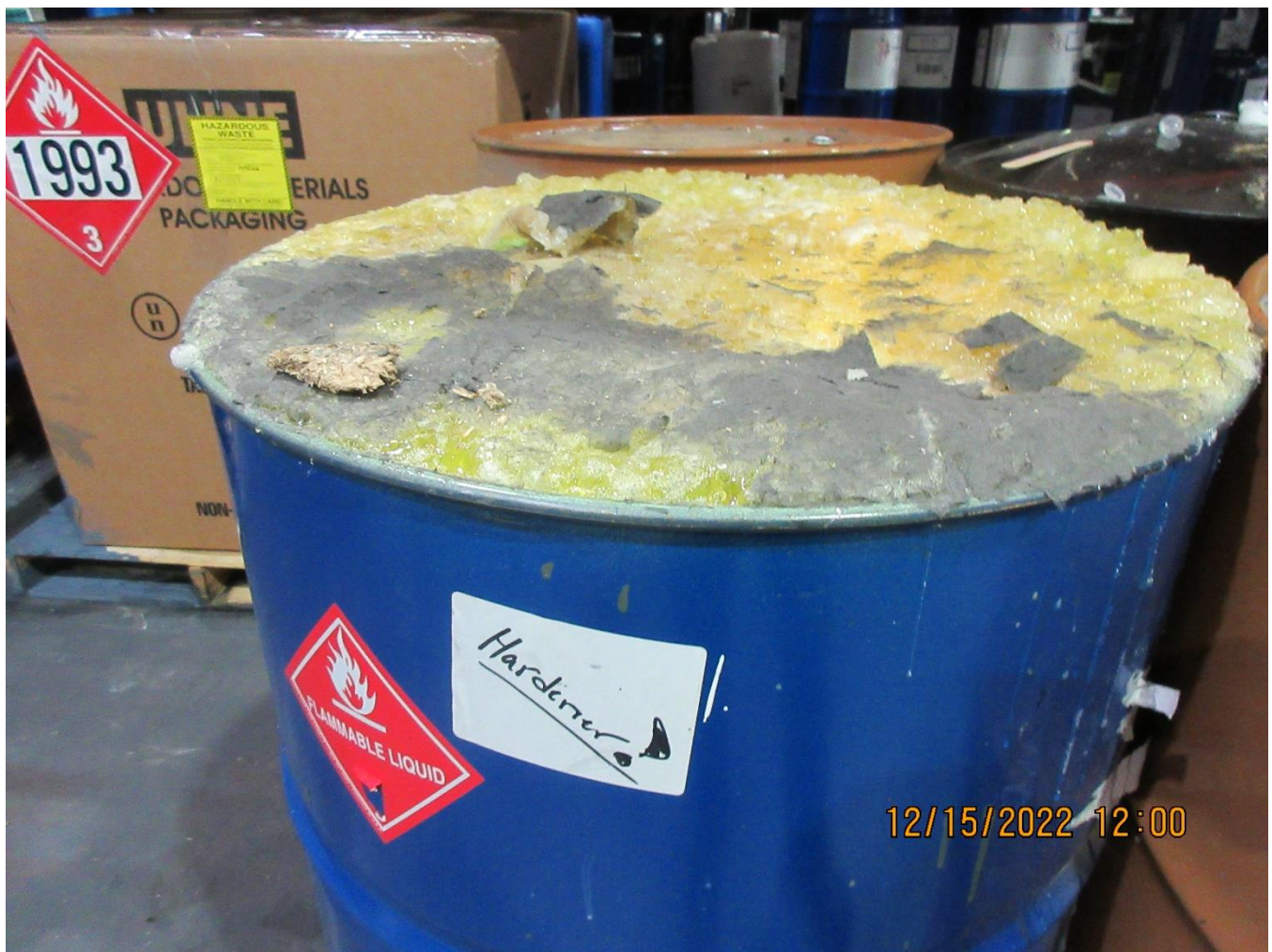
Photo 35 - Drum of Hardener with compromised lid in FLD drum position on pallet B4
