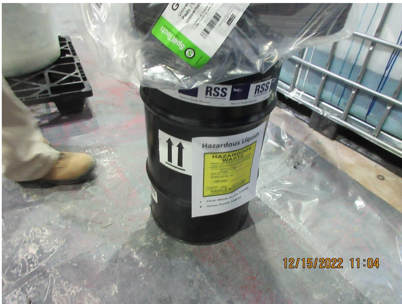
Photo 22 – 15-gallon container of hazardous waste liquids in central area of cleaning area w/o an accumulation start date.
