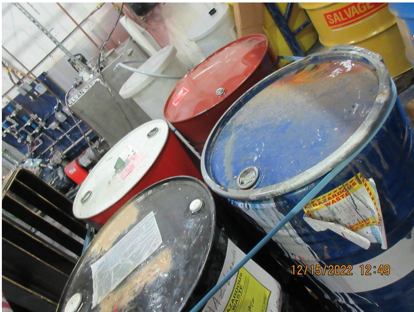
Photo 49 – Drums on pallet in T2 pallet position. Bung missing on bulging drum in BRD drum position on pallet in T2 pallet position
