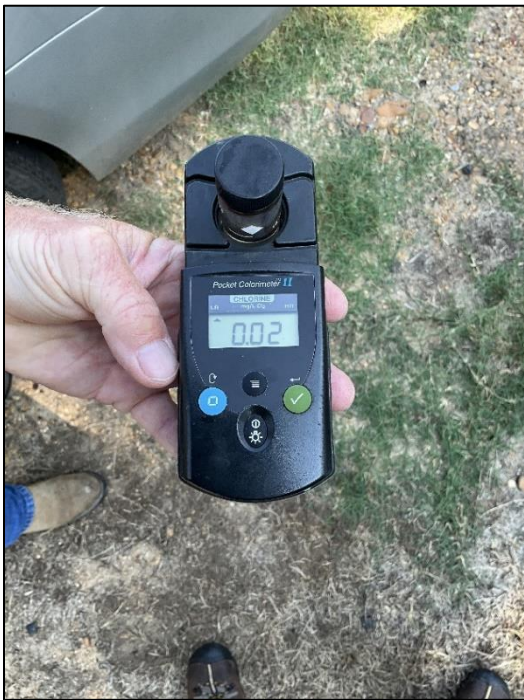
Photo 3: Residual Chlorine reading of 0.02 mg/L.
