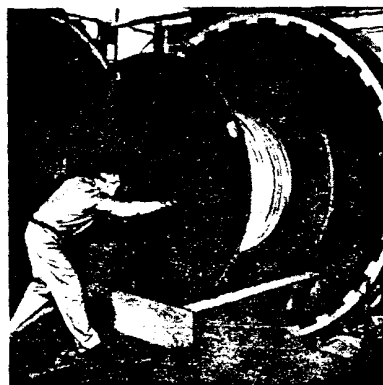
A spool of lead-encased reinforced- rubber hose being moved into a vul- canization oven. The oven is steam- heated to approximately 300°F.
