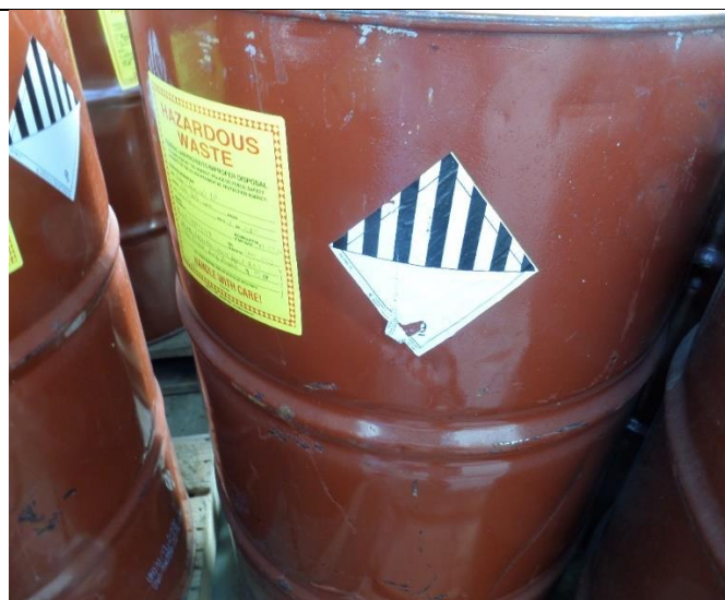
East Side of Building 130, CAA. Observed nine containers labeled with a #9 hazard indicator, not an indication of the hazard in the containers. Photograph 2 taken at 11:24 a.m.
