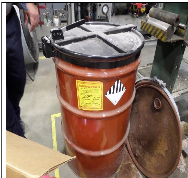
Building 130, Mechanic Shop. Observed the containers was labeled with a #9 hazard indicator, not an indication of the hazard in the container. Photograph 9 taken at 11:44 a.m.
