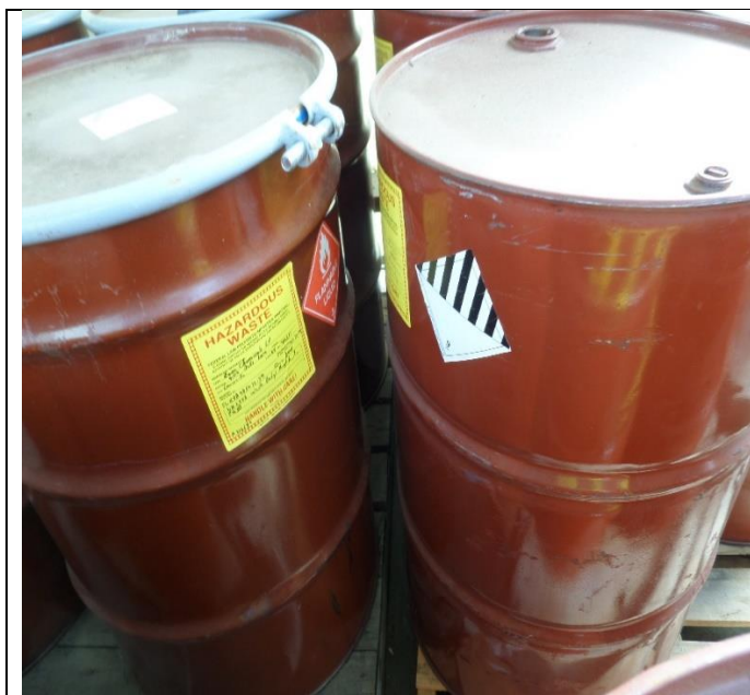
East Side of Building 130, CAA. Observed nine containers labeled with a #9 hazard indicator, not an indication of the hazard in the containers. Photograph 3 taken at 11:24 a.m.
