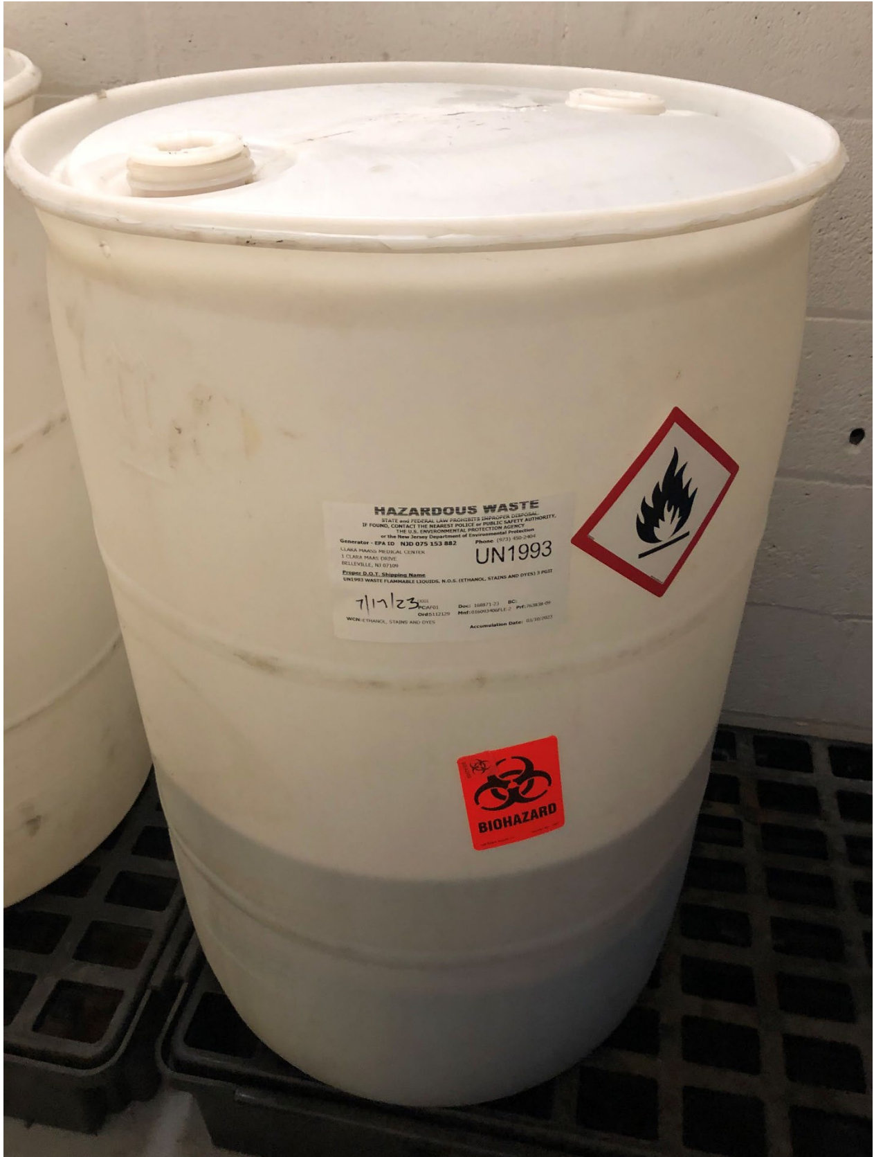
Photo #5: A 55-gallon drum of waste flammable liquids in the Hazardous Waste Accumulation Area.
