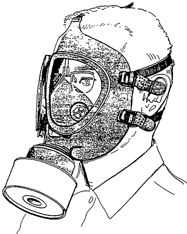
Fig. 3.8. Full face mask illustrating center mounted prescription glasses inside facepiece and nose cup insert.
