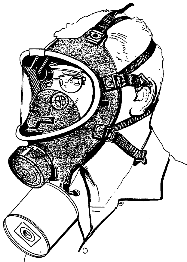
Fig. 3.10. Full face mask illustrating method of mounting prescription glasses inside facepiece with center mounted suction cup and nose cup insert.
