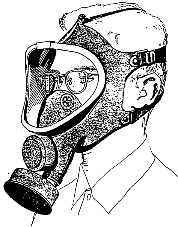
Fig. 3.9. Full face mask illustrating method of mounting prescription glasses inside facepiece by special mount on each side and nose cup insert.
