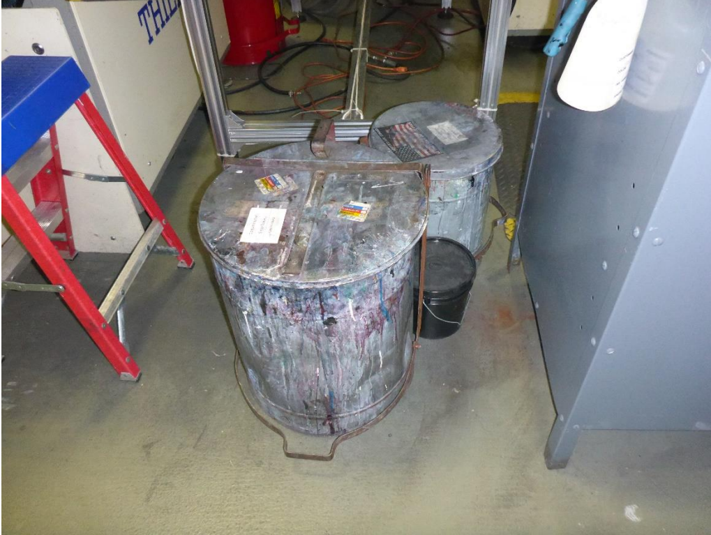
Photo 7: Flip-top containers for accumulating solvent contaminated wipes in the Screen Print Area Two. The containers were not labeled “excluded solvent contaminated wipes.”
