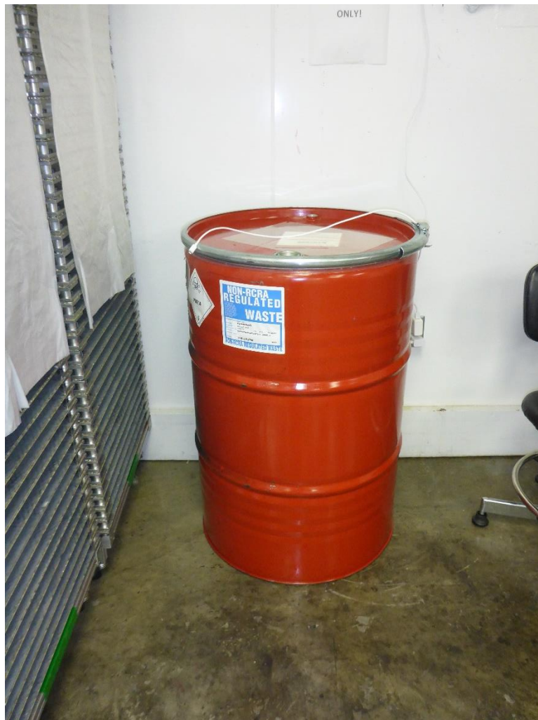
Photo 14: 55-gallon container labeled non-RCRA Isophorone diisocyanate in the Doming Area. The container was identified with a poison hazard placard and the waste profile number B107658.
