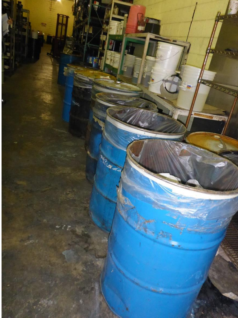
Photo 16: A row of six 55-gallon drums containing solvent contaminated rags in the Ink Shed. Five of the drums were labeled excluded solvent contaminated wipes, but the sixth drum was not labeled. Three of the drums did not have a lid, and the rings on two of the remaining three drums were not secured.
