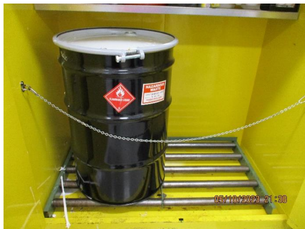
Photo 1: 55-gallon drum of polymer waste (Photo #1). The drum was properly closed, labeled with the words “Hazardous Waste”, and contained a flammable hazard indication.
