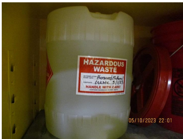
Photo 3: One 5-gallon closed container of hexane and methanol waste dated May 01, 2023, with a hazard indication for flammability.
