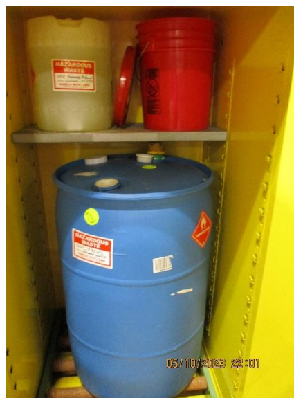
Photo 4: One 55-gallon closed drum of hexane waste. The container was dated April 26, 2023, with a hazard indication for flammability.
