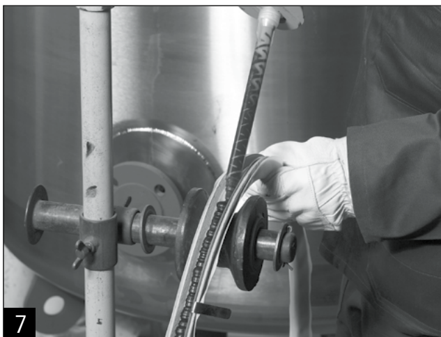
Press trigger on air gun. The ejection speed can be adjusted at the pressure regulator (Fig. 1, item 4).
