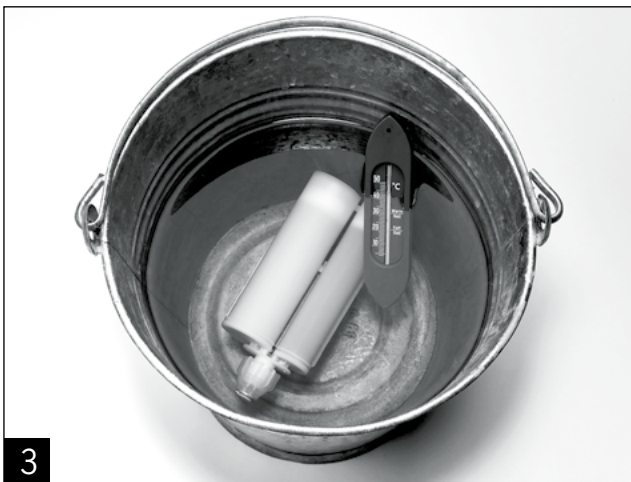
The temperature of the UF3000 filler material should be 40 \pm 10^\circ\text{C} when injecting the material. Warm up the filler material, if necessary (refer to Section 7.5).
