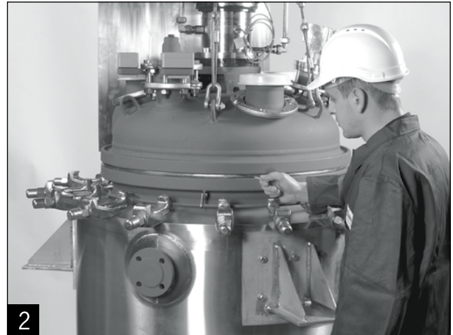
Placing cover in position on a trial basis. Use intermediate layer to protect the glass! Estimate gap width in order to determine the necessary quantity of UF3000.
