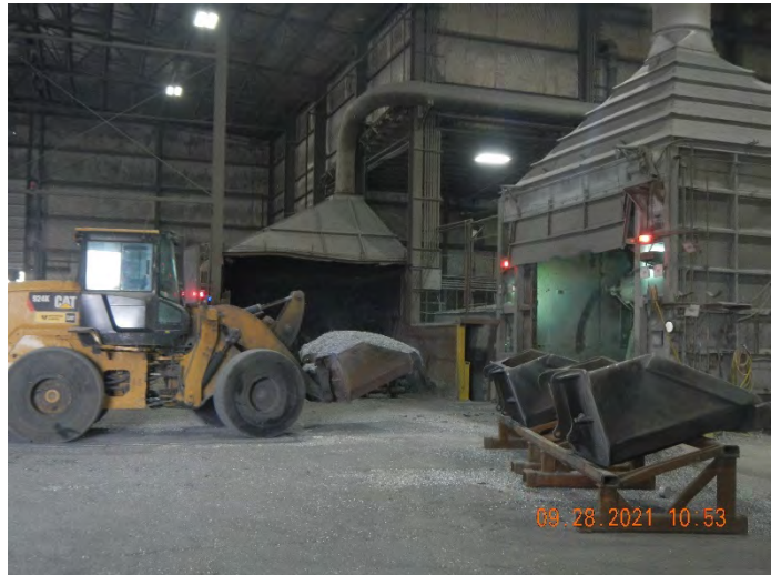
Photo #:04 (DSCN2505) Description: Facing northeast, photo of a loader being weighed prior to adding aluminum to Rotary Furnace #3.
