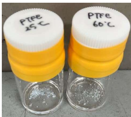
Figure 10: Pictures of electrolyte resistance test for PTFE, after 7days stored at 25°C (left), 60°C (right)
