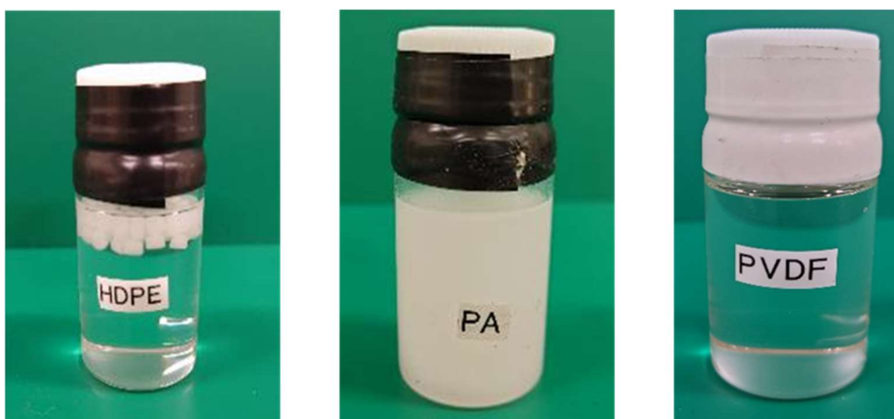
Figure 2: Picture of solubility test sample. HDPE (left, insoluble), PA (centre, insoluble), PVdF (right, soluble)
