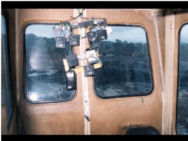
Figure 1. Interior cab sampling instrumentation on Ingersoll Rand drill.
