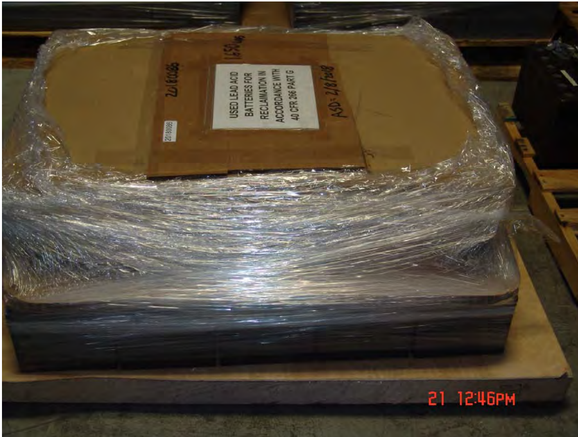
Lead acid batteries managed under 40 CFR 266 part G at the Hazardous Waste Management Center showing neatly stacked and shrink wrapped batteries.
