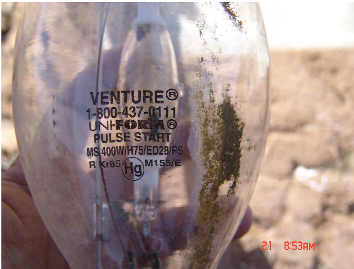
Used mercury vapor lamp found at the main post construction and demolition landfill close up.
