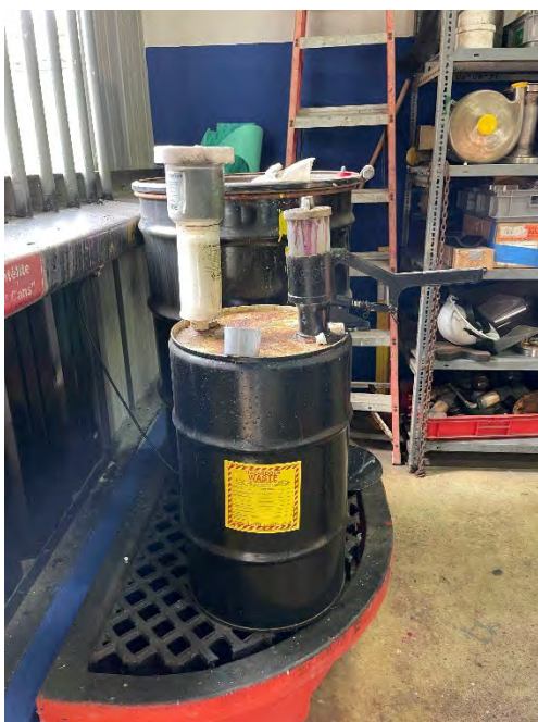
Photograph 3: Aerosol and Welding Shop SAA; 30-gallon drum of aerosol cans waste.
