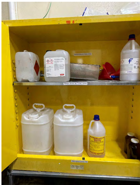
Photograph 1: F6 SAA; 5-gallon container of isopropyl alcohol not marked and/or labeled with the words “hazardous waste” nor with an indication of the hazards of the contents.
