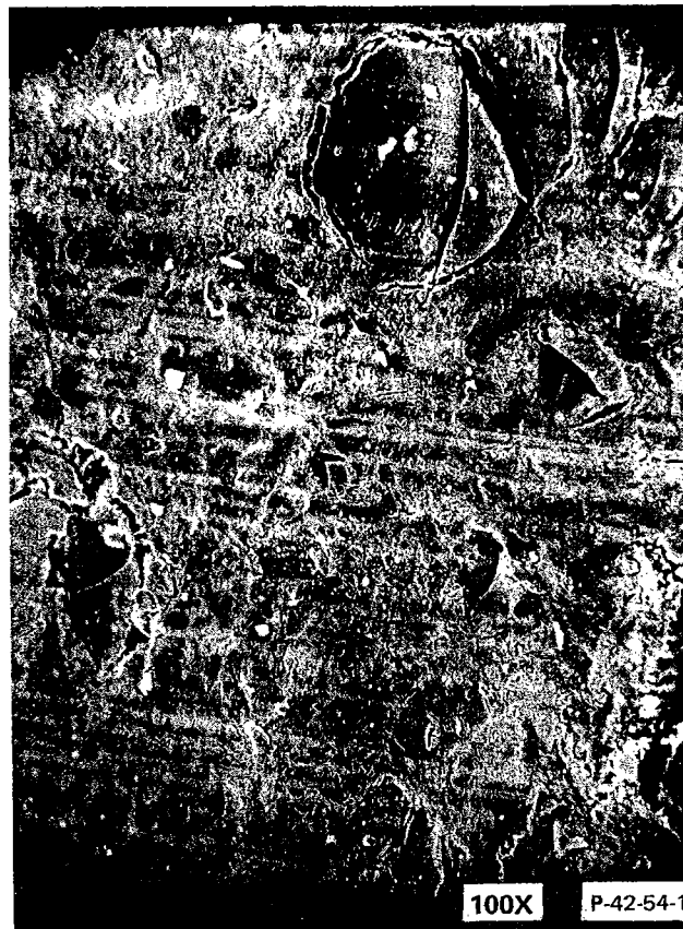
Figure 2-13 - Scanning Electron Photomicrograph Showing Abrasive Wear Tracks on Friction Material Surface and Adherent Wear Debris Particles
