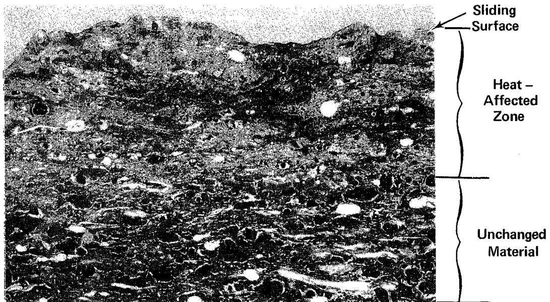
Figure 2-7 - Photomicrograph of Cross Section of Friction Material Test Specimen After More Than 10 Successive Stops from 100 mph on Bendix Full-Brake Dynamometer
