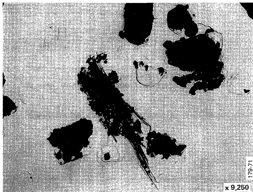
Figure 2-5 - Electron Micrograph of Friction Material Wear Debris (Made during 1966 studies) - 10,000 X
