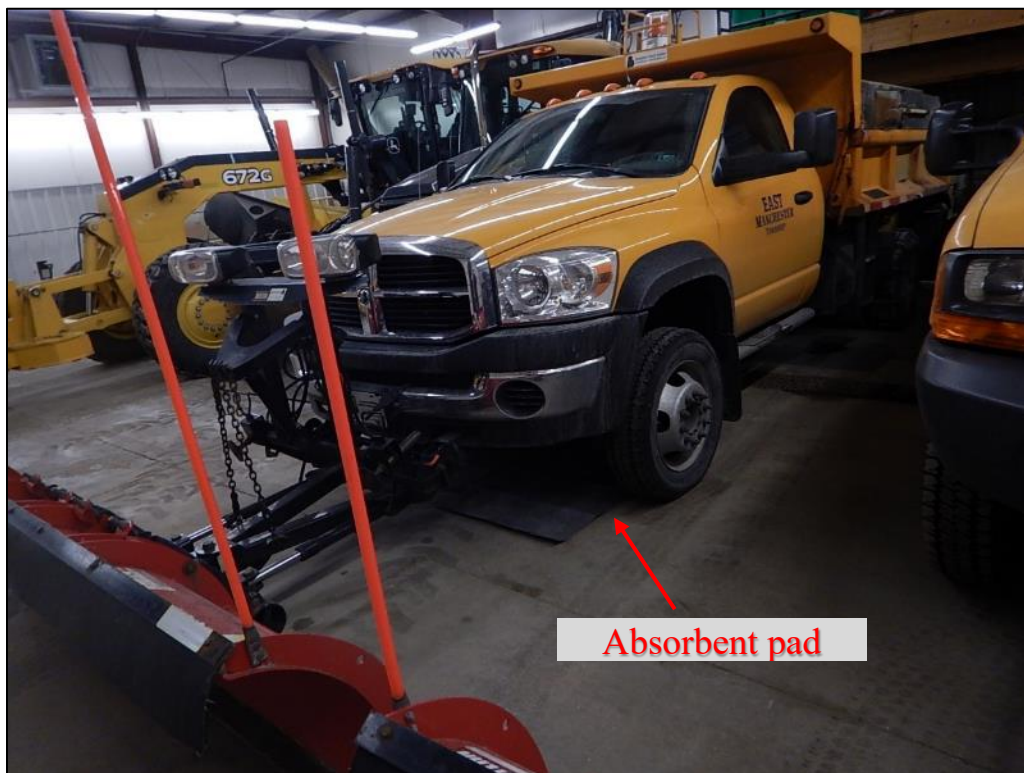
Photograph 14. View of the absorbent pads under the hydraulic line on a stored vehicle in the garage.
