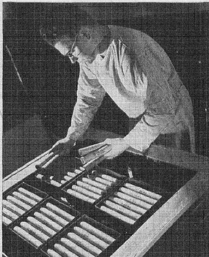
RIGHT: A moisture cabinet. Explosives are tested under varying conditions of temperature and humidity to simulate exposures that may be encountered in shipment and storage.
