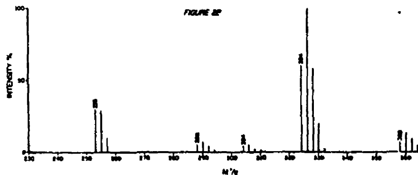
Figure 2B Mass spectrum resulting from GC-MS analysis of Fraction V 25% Et 2 O/Hex of Aroclor 1254 R . LKB 9000 GC-MS, other conditions see fig. 2A. Instrument calibrated with PFK.
