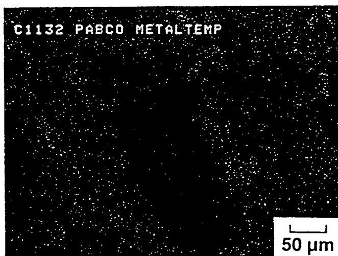
Pabco Metaltemp Board Showing Unreacted CaO Particle. (Top Photo: SEM Image, Middle: Ca Map, Bottom: Si Map)
