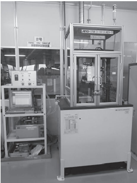
Photo 2. Ring-on-disk friction and wear test equipment
