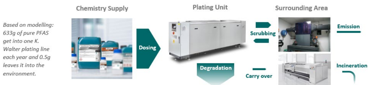
Figure 4: Material flow analysis of PFAS ([REDACTED]) in the hard Chrome plating process
