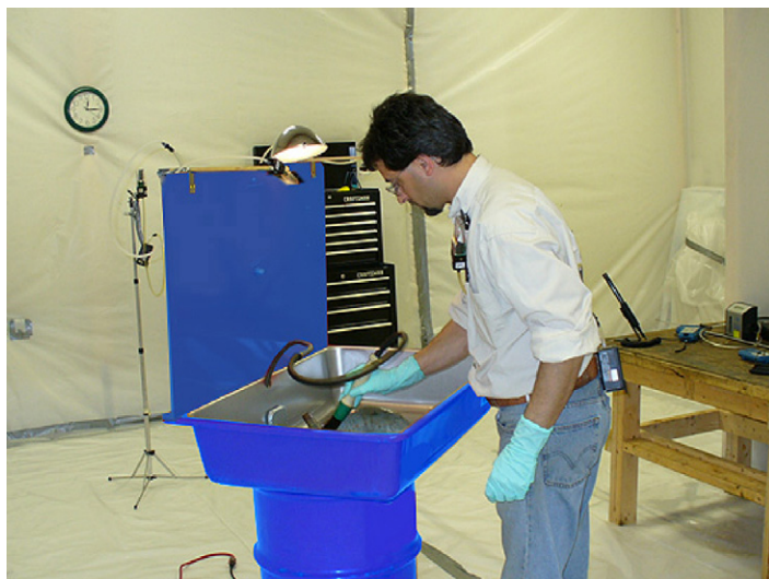
Plate 2. The parts washer apparatus used during Study #2. Note air samplers located at the top of the lid (NF zone) and on the tripod stand in the background (FF zone).
