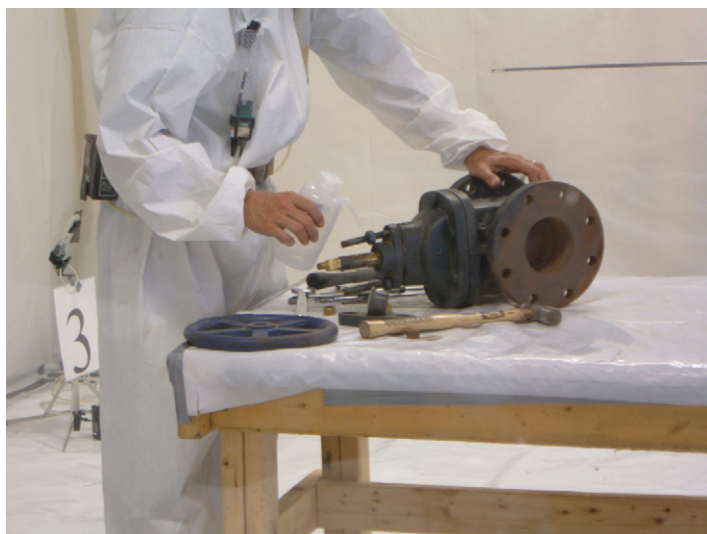
Plate 1. Cyclohexane being applied to gate valve during Process #1 trials.
