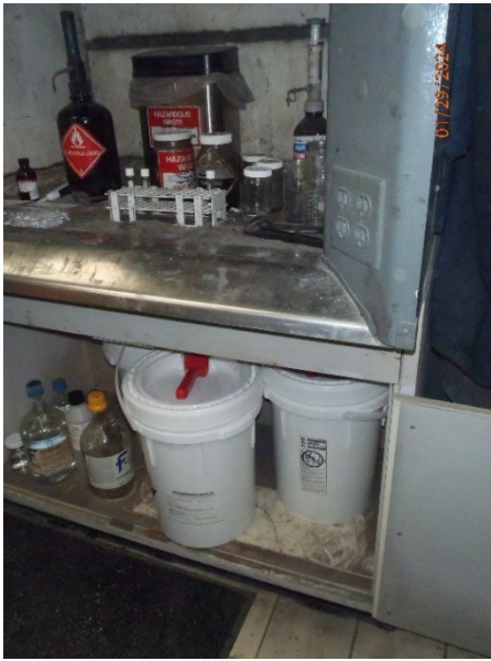
Picture 52 – Laboratory SAA containers
