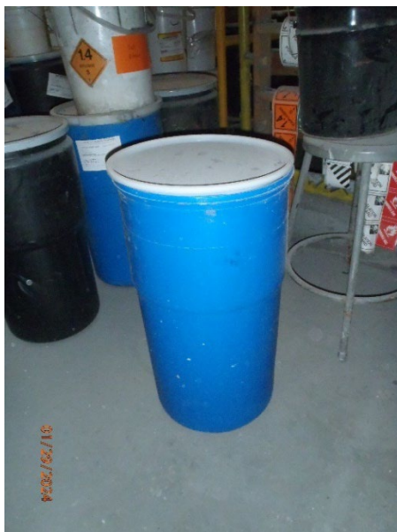
Picture 47 – Upper Warehouse Container Storage F open and unlabeled drum
