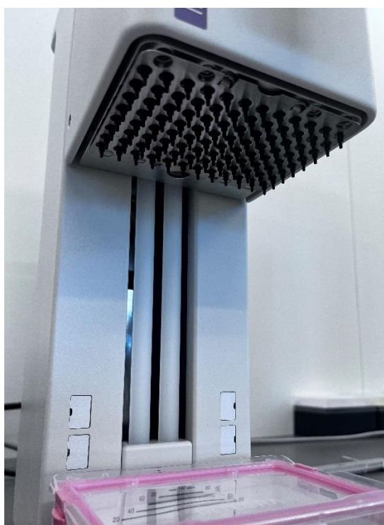
Figure 4-3 Example of fixed tips in liquid automation.
