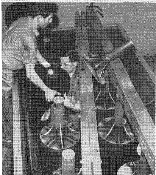
Dyed "tops" are lifted from kettle. New method now makes vat-dyed wool feasible.
