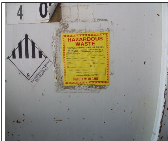
Central Tank Farm. The inspector observed the 3,250-gallon vacuum truck not marked with a toxic hazard indicator. Photograph 7 taken at 10:29 a.m.
