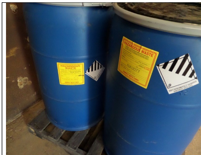
Waste Pile Building #2. 90-Day Area. The inspector observed two 55-gallon containers of hazardous waste without a toxic hazard indicator. Photograph 1 taken at 10:18 a.m.
