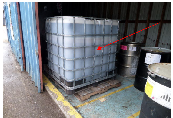
Photo-5 275-gallon tote containing waste sludge (D008)
