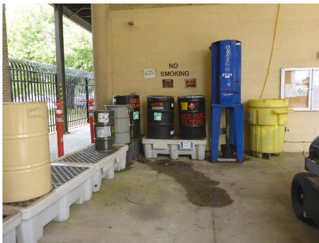
Photo 14: 35-gallon container for accumulating used sumpens in a SAA at the 403 rd Aerospace Ground Equipment Area, and one 55-gallon container for accumulating hazardous waste used fuel filters in another SAA at the 403 rd Aerospace Ground Equipment Area.
