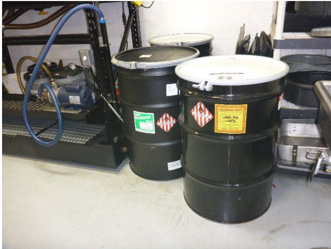
Photo 10: Two SAAs at the Building 4430 Vehicle Maintenance Area. One 55-gallon container for accumulating hazardous waste absorbent materials used to clean gasoline spills or leaks in one SAA. One 55-gallon container for accumulating hazardous waste pig-mats used to clean spills and leaks that are not gasoline in the second SAA.
