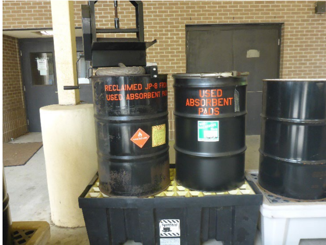
Photo 13: 55-gallon container for accumulating hazardous waste Jet A/JP-15 in a SAA at the 403 rd Aerospace Ground Equipment Area.
