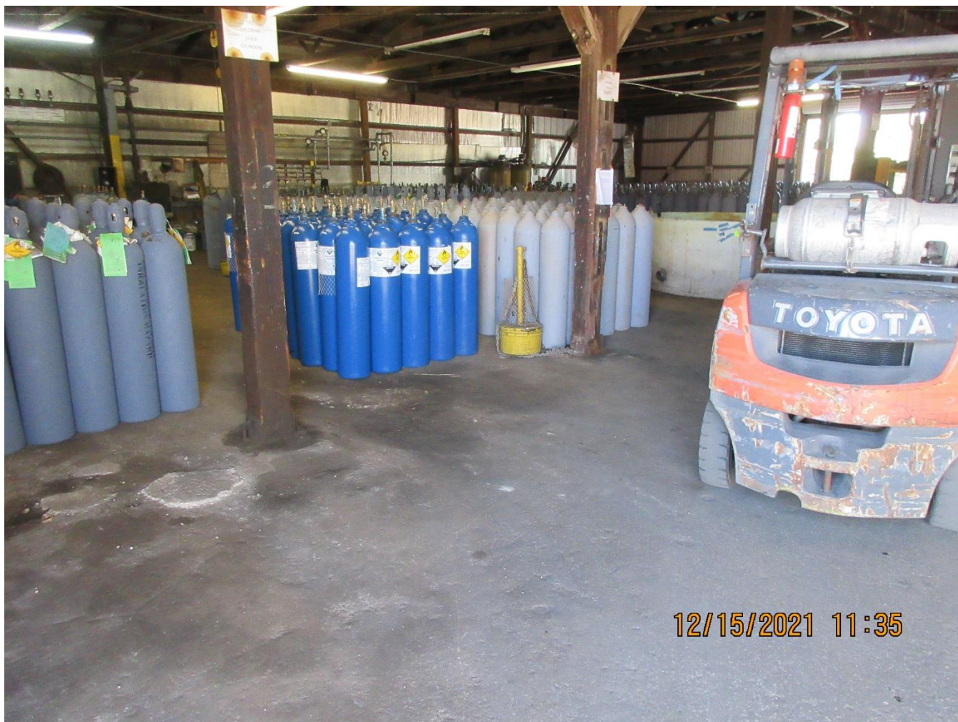
Photo 19 – 150 Pound Chlorine Containers
