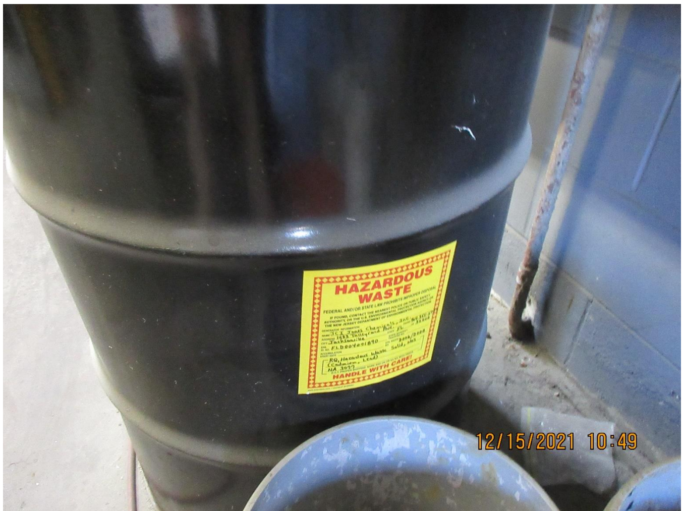
Photo 7 - Glass bead media blast unit hazardous waste container
