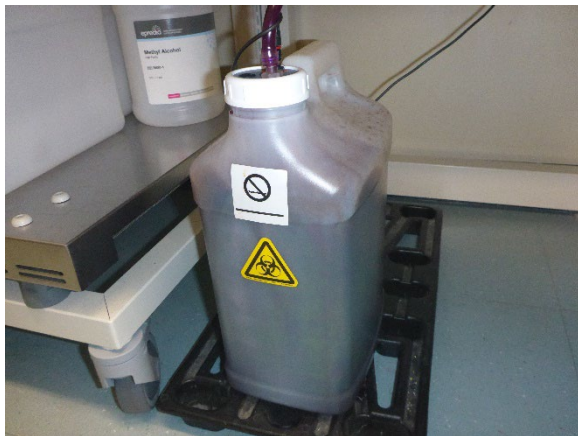
Photo 3: 2.5-gallon container accumulating gram stain hazardous waste in the Microbiology Laboratory SAA. The container is marked to indicate that the contents pose a biological hazard, but it is not marked to indicate that the contents are flammable.
