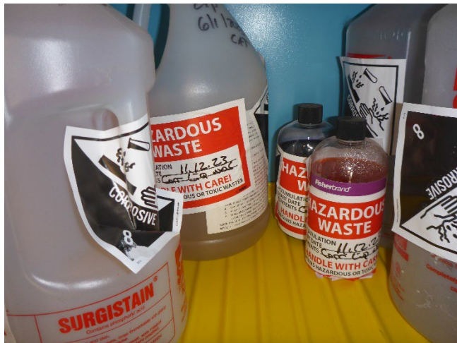
Photo 30: Containers of waste corrosive liquids inside the acid cabinet at the CAA. Each container appeared to be labeled with the words "Hazardous Waste", identified with an indication that its contents are corrosive, and marked with an accumulation start date.
