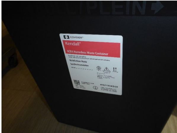
Photo 10: The 18-gallon container was labeled with the words "Hazardous Waste", but it was not marked with an indication of the hazards of its contents.
