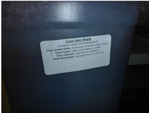
Photo 2: Label on 2.5-gallon container of gram stain hazardous waste in the Microbiology Laboratory SAA. The label indicates that the gram stain waste contains ammonium acetate, ethyl alcohol, isopropyl alcohol and acetone.
