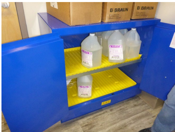
Photo 15: Corrosive cabinet in the Dialysis area to hold 1-gallon containers of leftover product, which is characterized as D002 hazardous waste.
