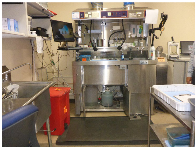
Photo 8: One of two stations where formalin is used with specimens at a vented laboratory sink. The inspectors observed one container of clean formalin and one container of dirty formalin in the cabinet beneath the sink.
