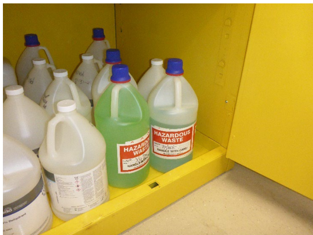
Photo 7: The second of two flammable cabinets used to hold containers of hazardous waste accumulated in the Pathology SAA. The inspectors observed several 1-gallon containers labeled waste in this cabinet. Three containers were labeled as hazardous waste and marked to indicate that its contents are flammable.
