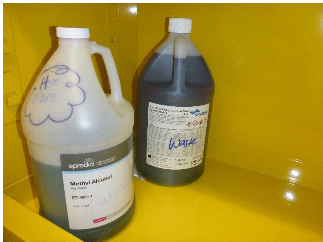
Photo 4: Two of three 1-gallon containers accumulating hazardous waste alcohols in the Chemistry / Hematology Laboratory SAA. Each container was labeled with the word “waste” and identified with the indication of hazards on the original labels, but they were not labeled with the words "Hazardous Waste".
