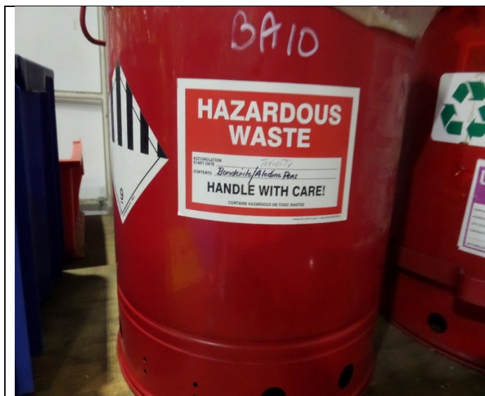
Building A. BA018 SAA. Observed one 10-gallon container not marked or labeled with a hazard indicator. Observed BAE representatives marked the container with the word toxicity. Photograph 1 taken at 11:04 a.m.
