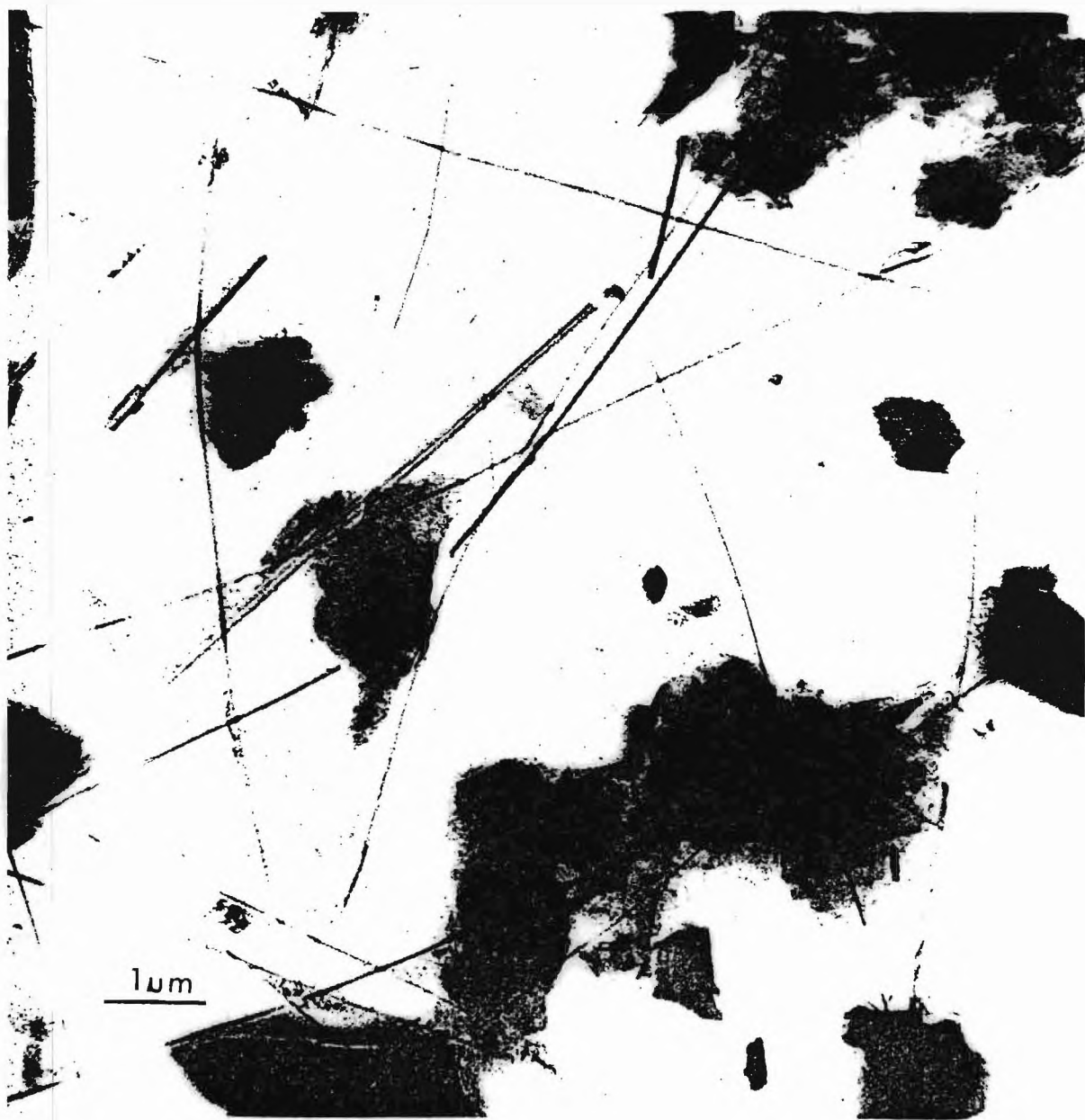
FIGURE 3. Electron photomicrograph of chrysotile-talc (95% talc, 5% chrysotile).
