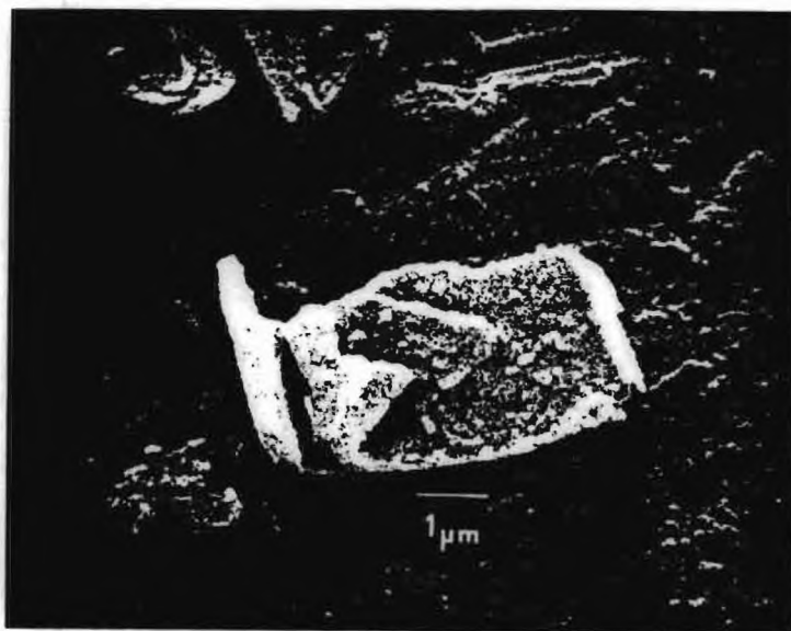
Figure 4. This micrograph illustrates the morphology of a typical curved talc platelet. The problems associated with attempting to define a fibrous structure by optical microscopy and its limited depth of focus can be seen. The optical microscope would make the above particle appear to be two separate particles, one of which would appear as a fiber and the other as a platelet.
