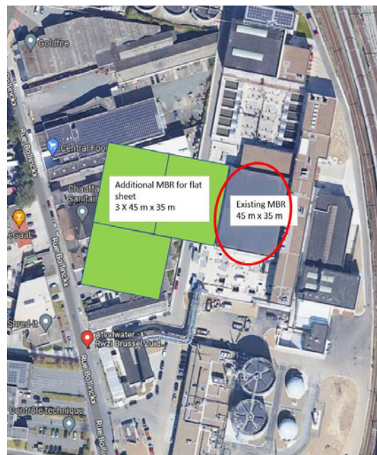
FIGURE 18: PRESENTATION OF ADDITIONAL LAND REQUIREMENT FOR FLAT SHEET POLYMERIC IN COMPARISON TO EXISTING MBR WITH [REDACTED] IN BRUSSELS.
