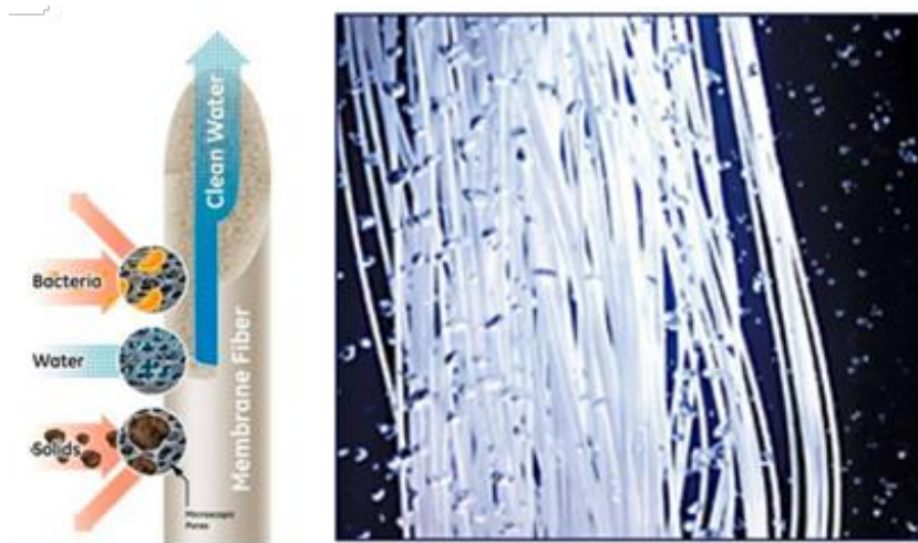
FIGURE 3: HOLLOW-FIBER MEMBRANE STRING (LEFT), ARRANGEMENTS OF STRINGS (RIGHT).
