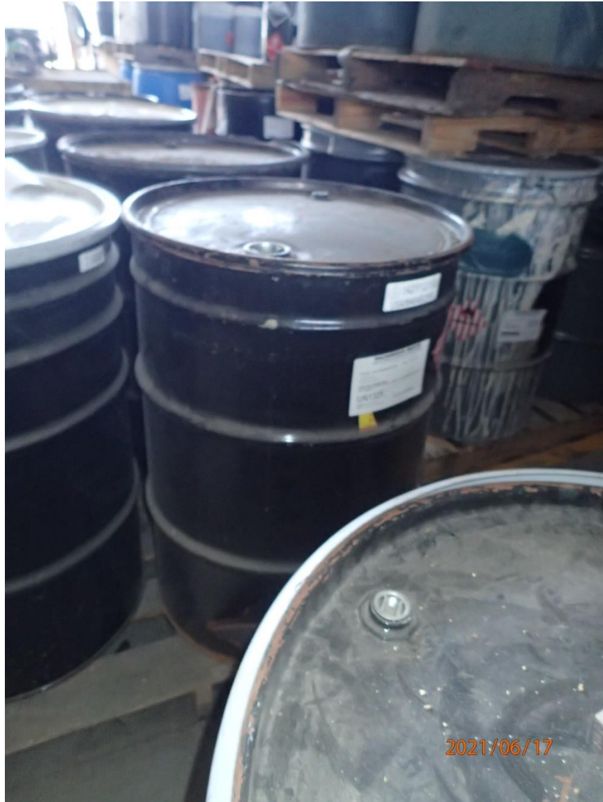
Photo 16: One of eight 55-gallon containers not properly closed, missing locking ring.
