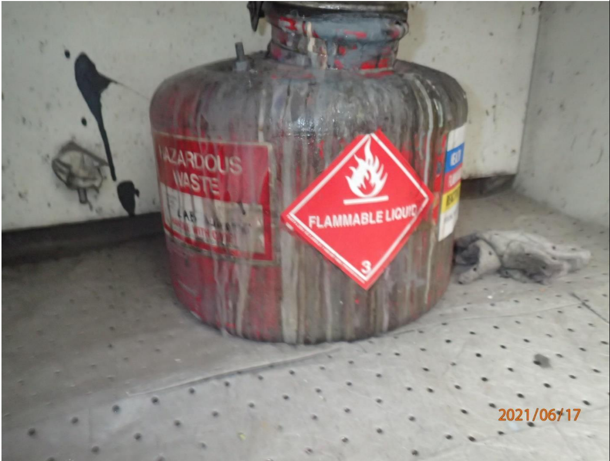
Photo 3: 5-gallon container of lab sample waste under a fume hood labeled “Hazardous Waste”, closed, and with an indication of hazard for flammability
