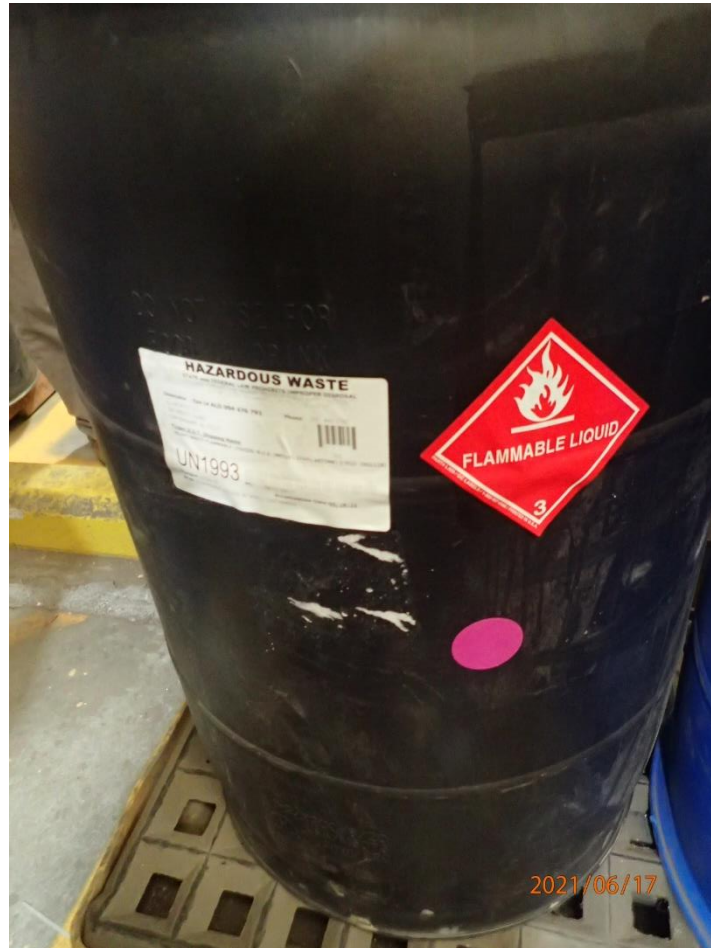
Photo 4: 55-gallon drums of laboratory waste on spill containment pallet labeled “Hazardous Waste”, closed, dated, and with DOT placards to indicate the hazardous contents.
