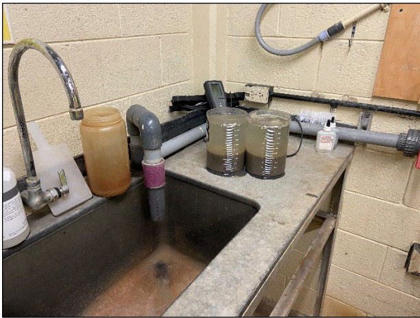
Photo 5: Settleometer testing station.
