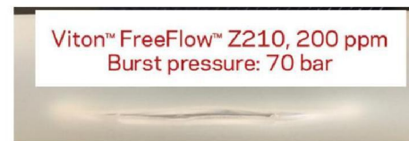
Pipe extruded with Viton™ FreeFlow™. Smooth inner and outer surface, improved concentricity, gauge and positive effect on material properties.
