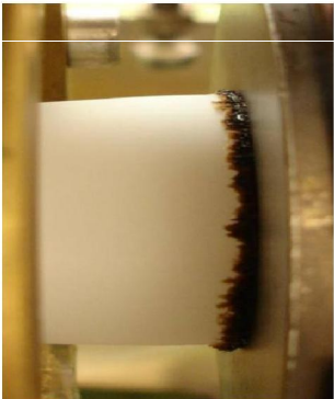
Die build-up formation after 1 hour extrusion without PPA
