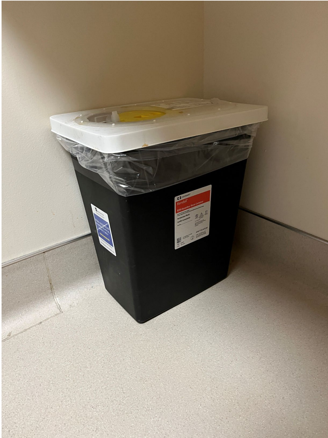
Photograph 3: 8-gallon hazardous waste satellite containers located in IV room for pharmaceutical waste
