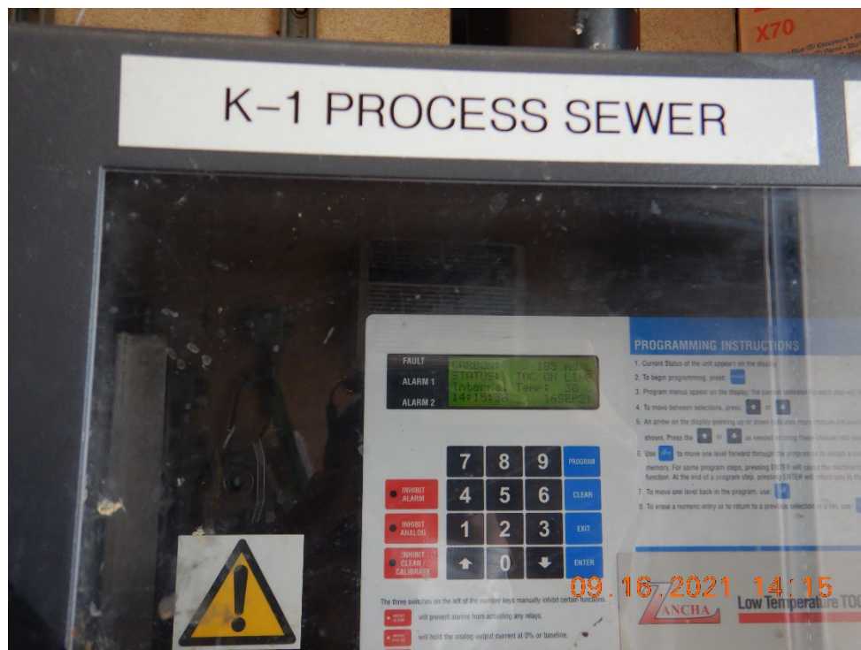
CWA Photo 4. View of the K1 TOC analyzer, which read 185 mg/l (ppm) at the time of the sampling on 9/16/2021.
