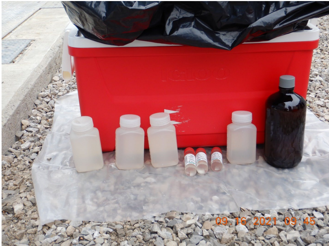
RCRA Photo 33. A view the grab sample (SP-2) taken directly from sample tap into sample containers held by sampler. The sample tap was flushed prior to sample being taken. Sample was clear liquid and no visible solids.
