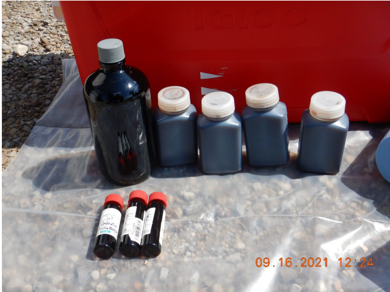
RCRA Photo 41. A view of grab sample (SP-6) taken directly from tanker trailer using a coliwasa to allow for a representative columnar sample of all material the tank. Sample was black liquid with no visible solids.
