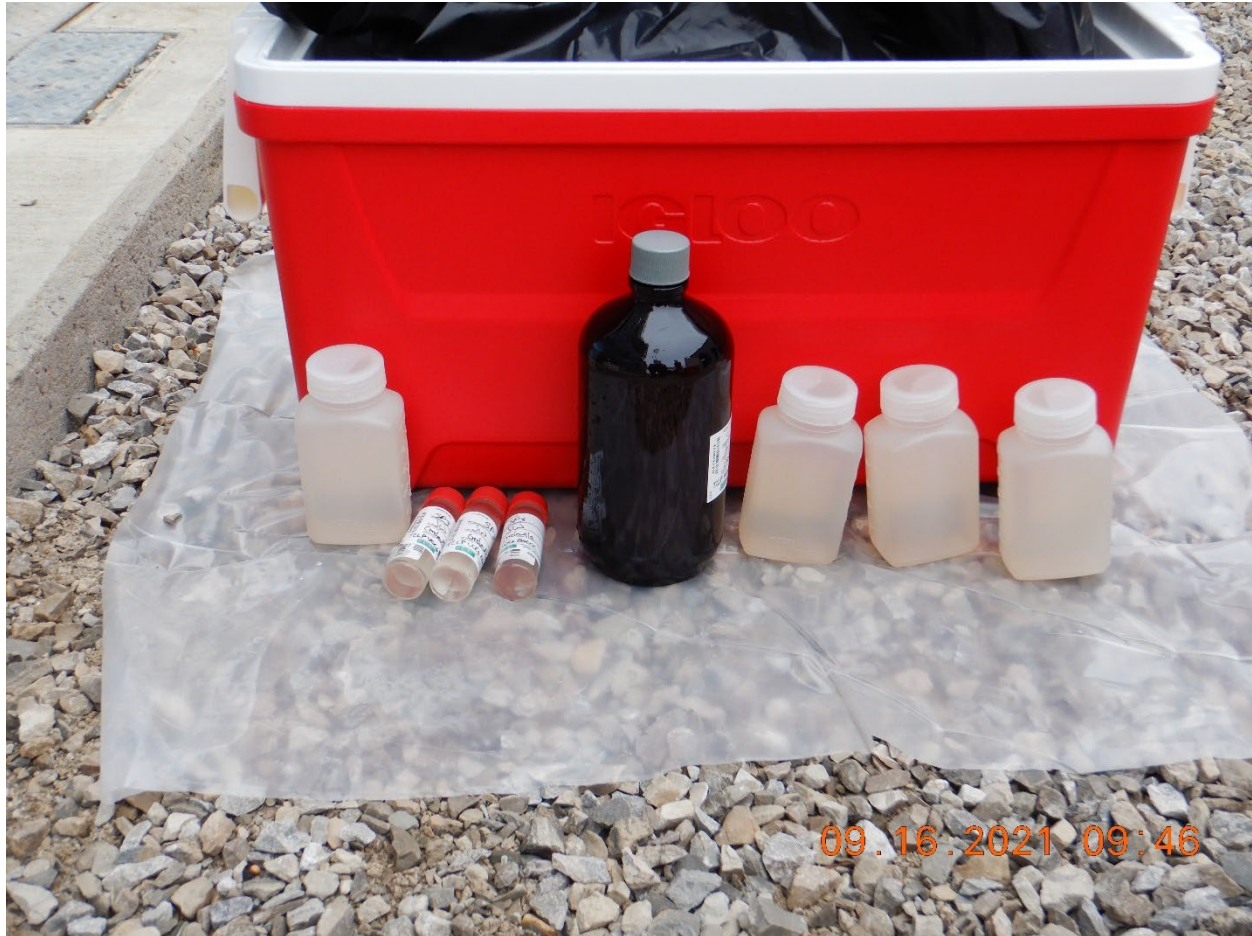
RCRA Photo 35. A view of grab sample (SP-3) taken directly from sample tap into sample containers held by sampler. Tap was flushed prior to sample being taken. Sample was clear liquid and no visible solids.
