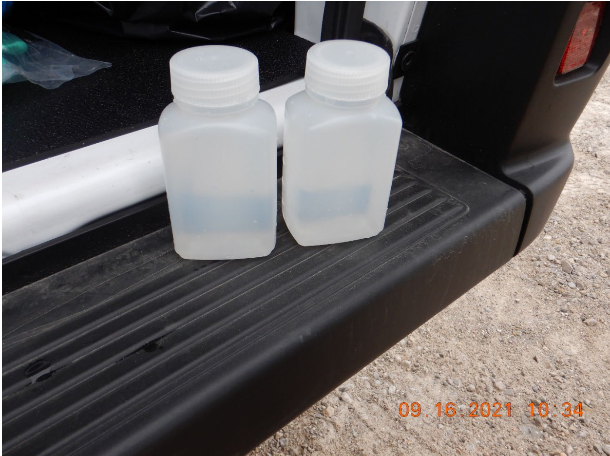
RCRA Photo 38. A view of the fluorocarbon chemical equipment blank (SP-4) taken prior to sampling the tanker trailer shown in Photo 37.
