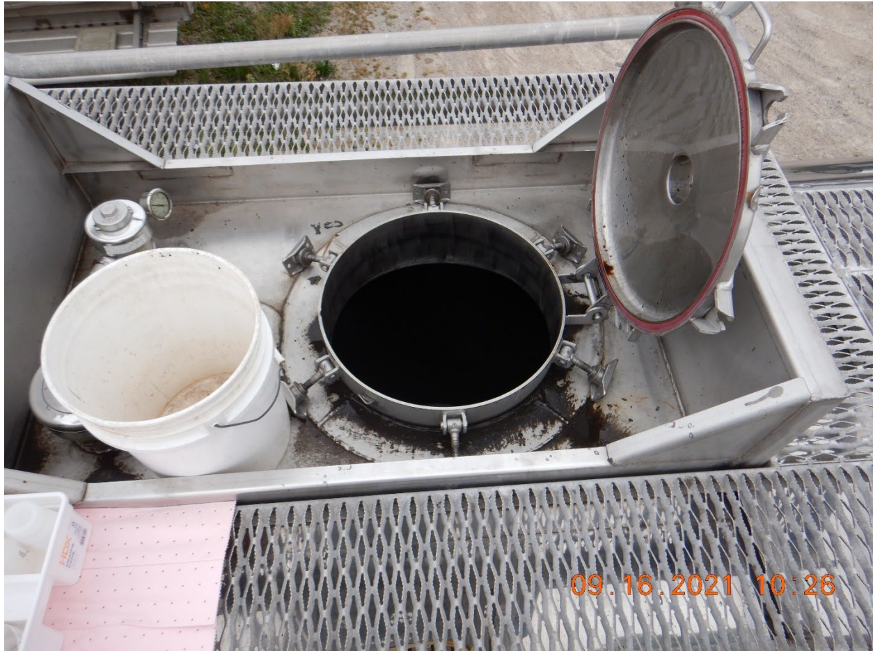
RCRA Photo 37. A view of the open manway cover on tanker trailer LT-1625 prior to sampling.
