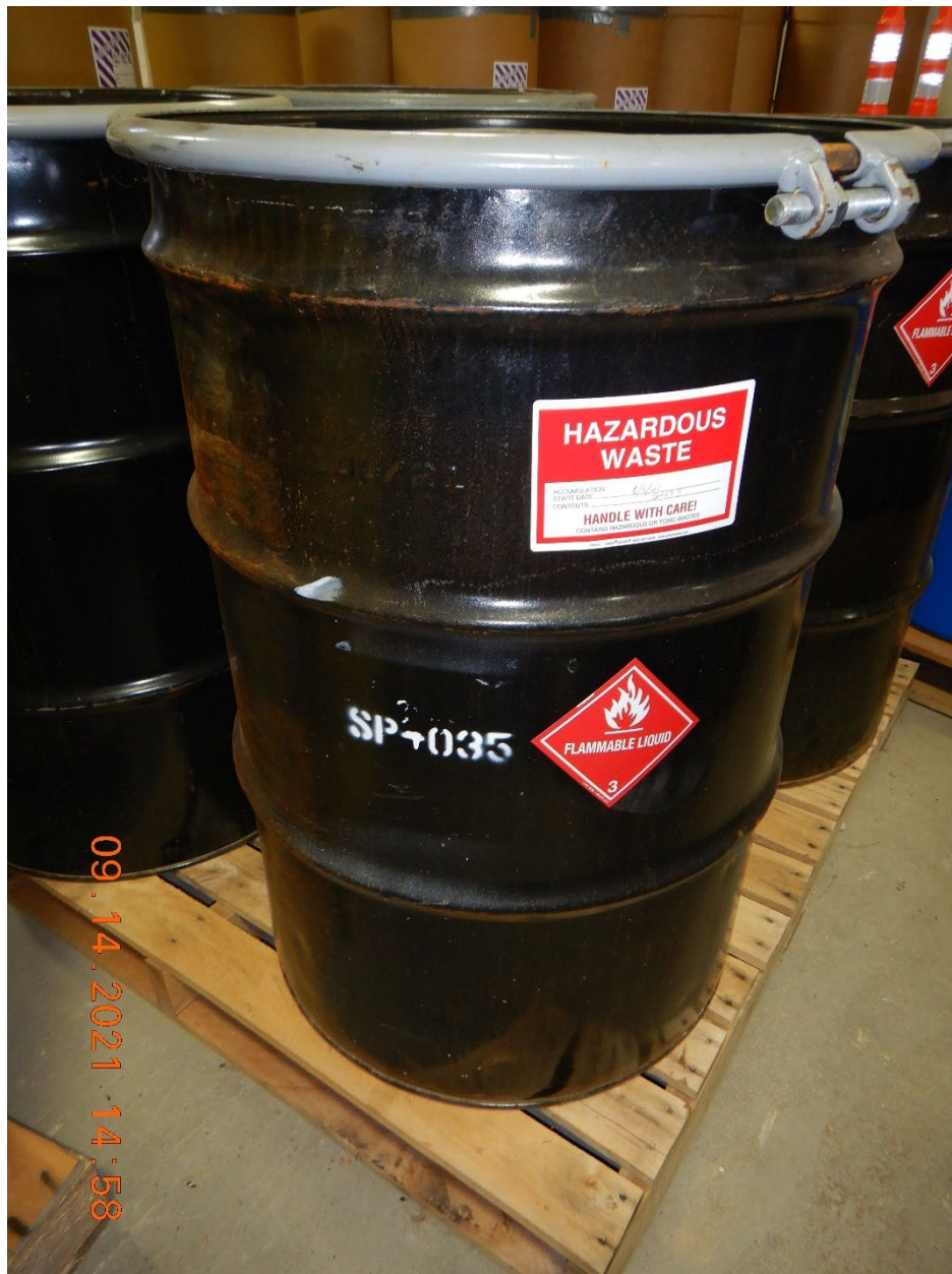
RCRA Photo 17. A view of one of four 55-gallon hazardous waste containers located in the facility's Building 510 CAA. The containers had an accumulation date of "6/30/2021". This date is over the 90-day accumulation limit for the facility's CAA.
