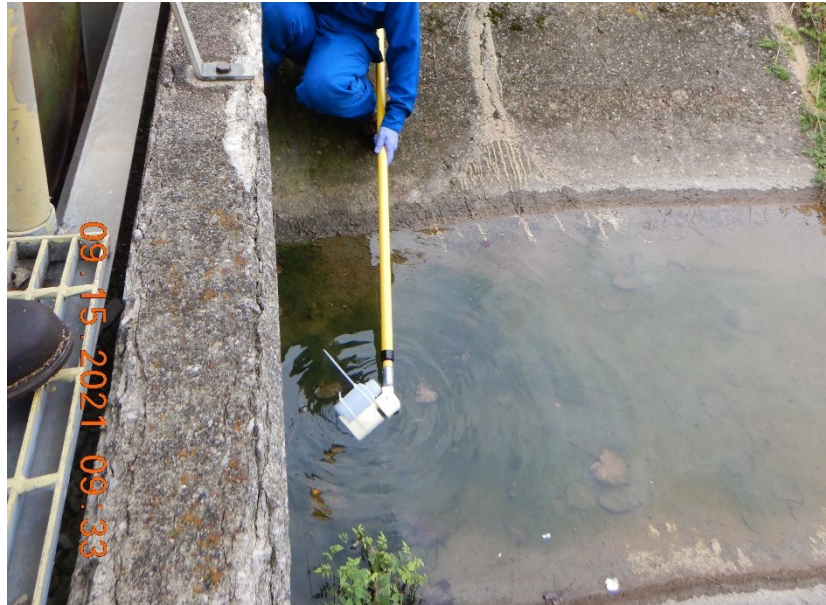
CWA Photo 22. View of sampling of the slowly flowing water in the concrete ditch use for stormwater and NCCW. This water was not discharging at the time of sampling.
