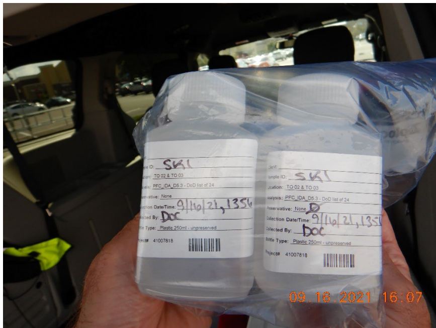
CWA Photo 34. View of the SK1 samples, which were clear with no visible solids.
