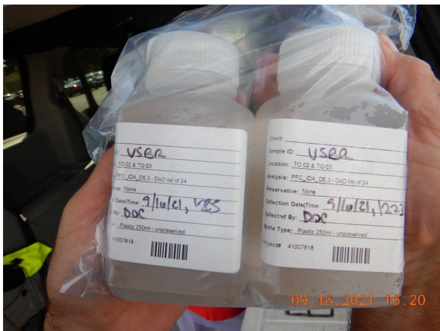
CWA Photo 28. View of VSBR samples, which were slightly brown with a small amount of solids.
