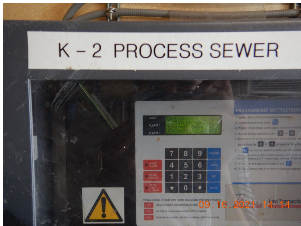
CWA Photo 6. View of the K2 TOC analyzer, which read 12 mg/l (ppm) at the time of the sampling on 9/16/2021. The time reading on this analyzer was off by 1 hour and 40 minutes.
