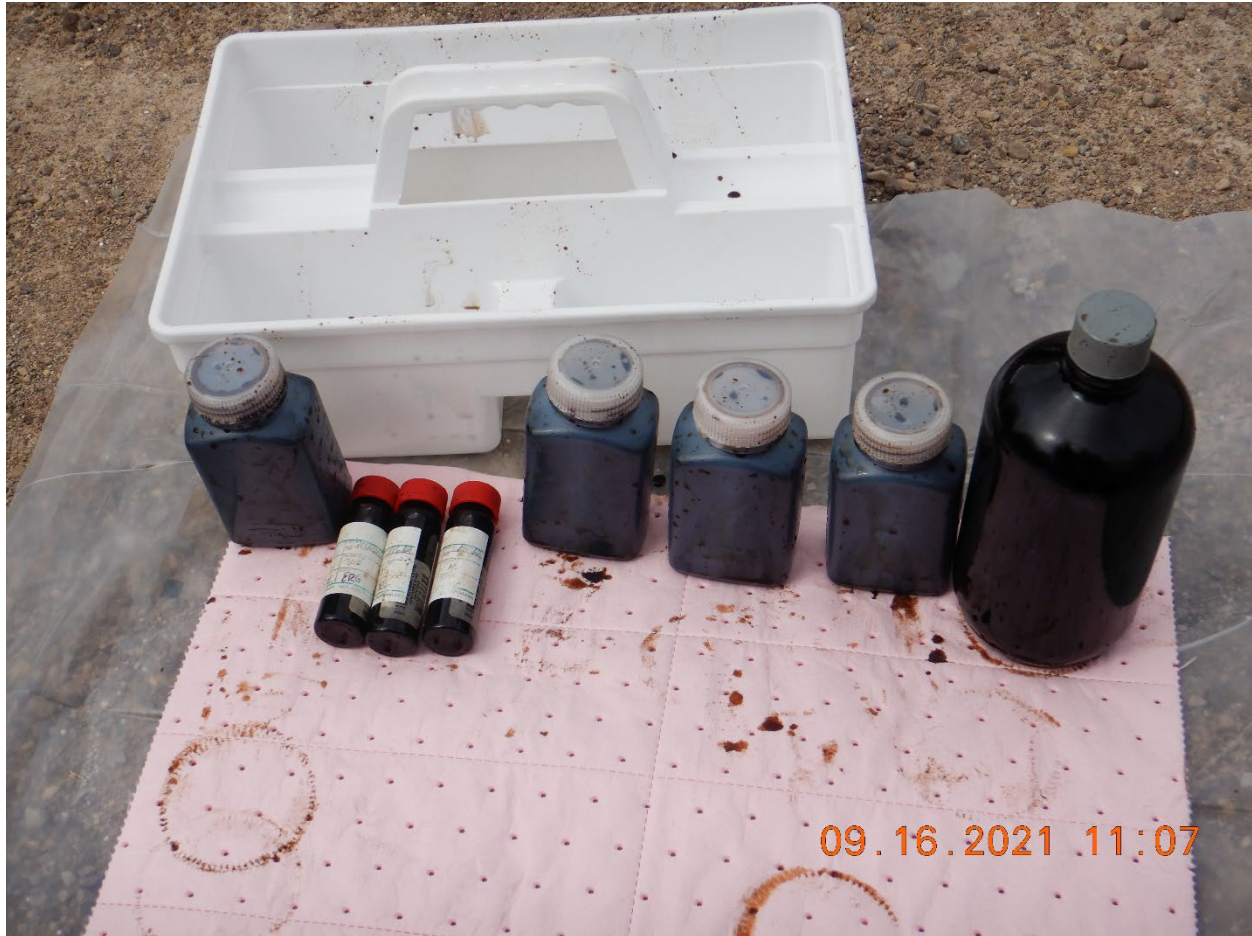
RCRA Photo 39. A view of grab sample (SP-5) taken directly from tanker trailer LT-1625 using a colliwasa to allow for a representative columnar sample of all material the tank. Sample was black liquid with visible flakey pea-sized solids.
