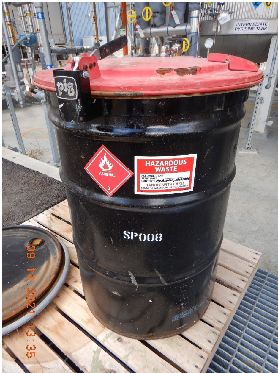
RCRA Photo 10. A view of a SAA 55-gallon container located near the hazardous waste tank used primarily to collect samples taken of rain water that is observed in the secondary containment area for the hazardous waste tank.
