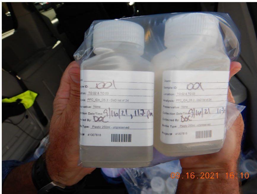
CWA Photo 32. View of 001 samples, which were clear with a slight brown tint.
