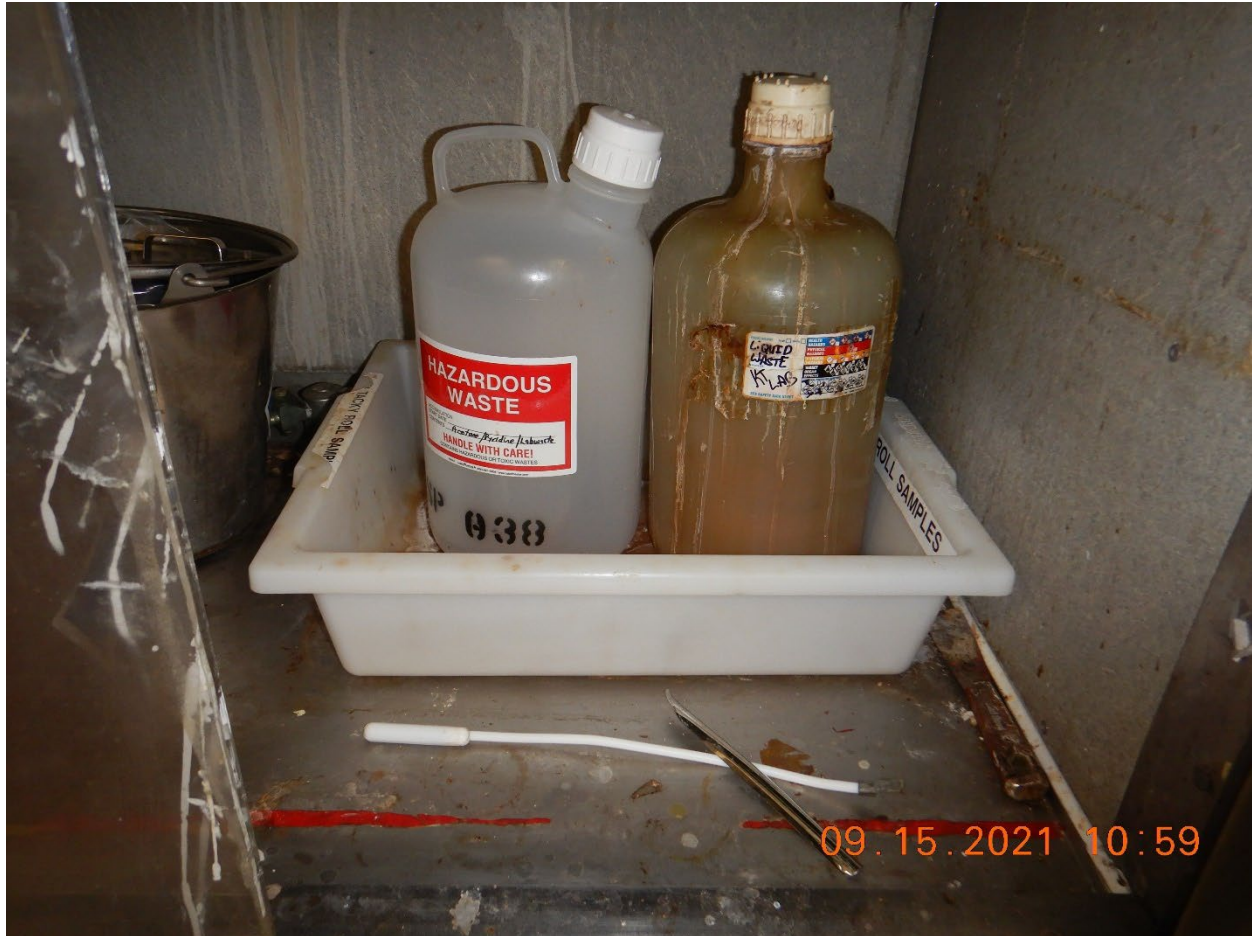
RCRA Photo 30. A view of hazardous waste that is stored inside the laboratory hood. The waste is then transferred from this SAA container into the SAA container shown in Photo 31.
