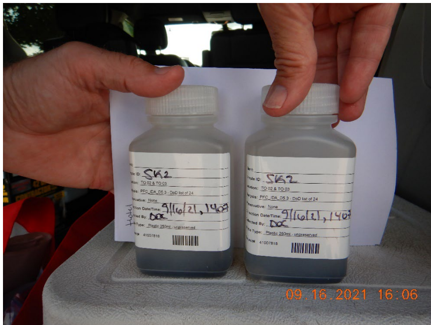
CWA Photo 36. View of the SK2 samples, which were clear with settleable black solids.
