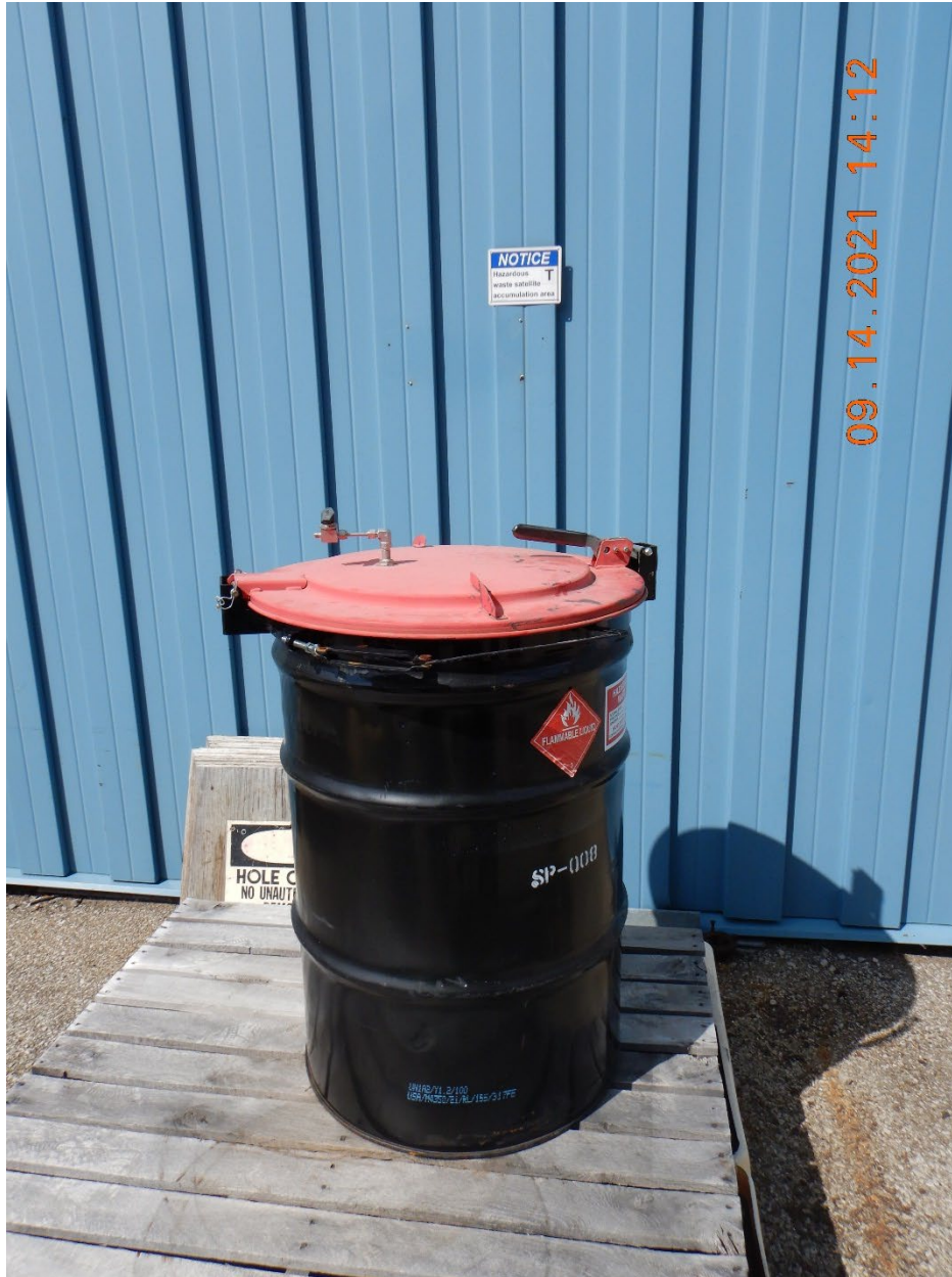
RCRA Photo 13. A view of a SAA 55-gallon container located outside of Building 2. The container holds process samples and drain helps from process tanks.
