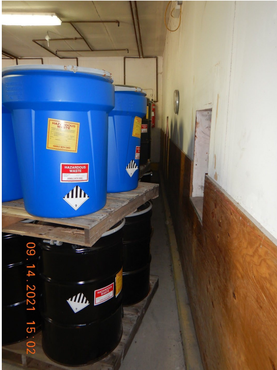
RCRA Photo 22. A view of the tight aisle space between hazardous waste containers located in Building 510 CAA.
