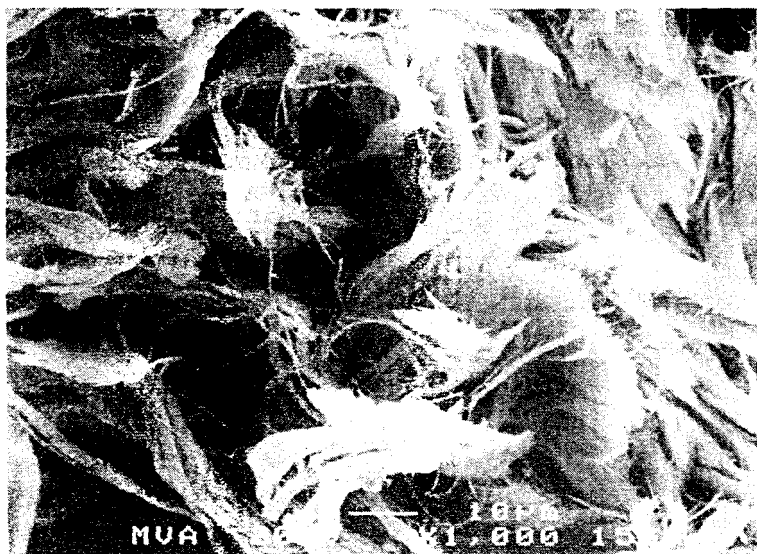
Figure 6-27. Close-up view of the surface of the gasket material shown in Figure 6-24 showing uncoated chrysotile asbestos fibers protruding.
