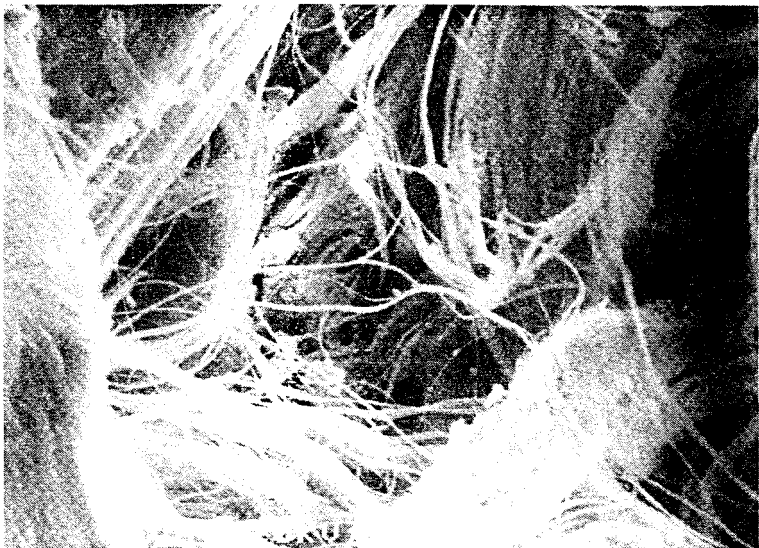
Figure 6-11. Close-up view of the surface of the gasket material shown in Figure 6-4 showing uncoated chrysotile asbestos fibers protruding.
