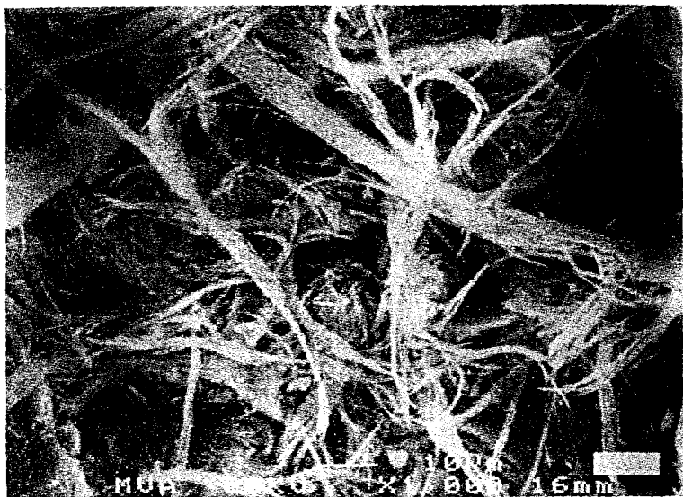
Figure 6-15. Close-up view of the surface of the gasket material shown in Figure 6-8 showing uncoated chrysotile asbestos fibers protruding.
