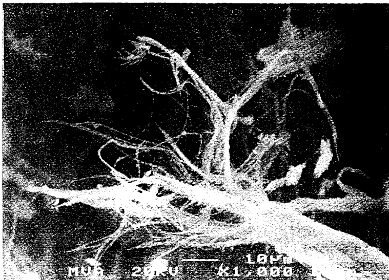
Figure 6-12. Close-up view of the surface of the gasket material shown in Figure 6-5 showing uncoated chrysotile asbestos fibers protruding.
