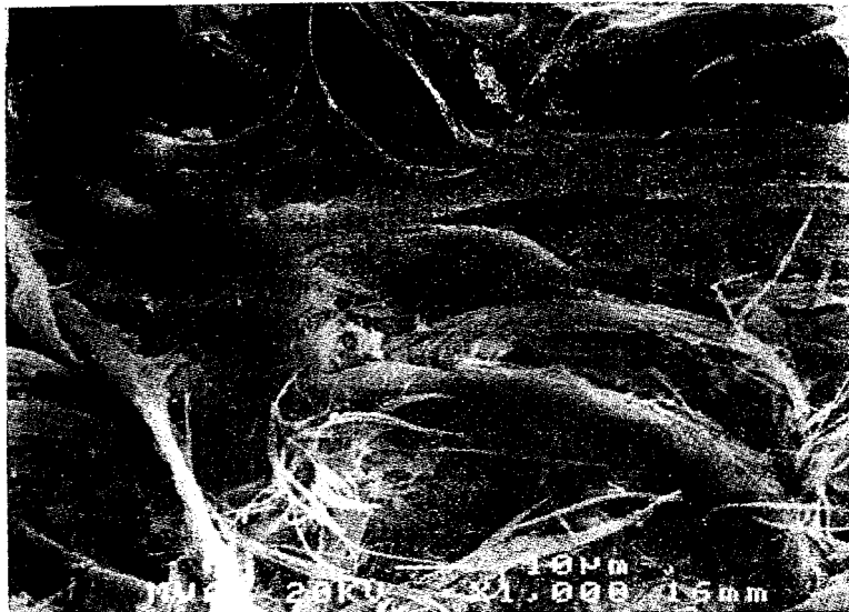
Figure 6-13. Close-up view of the surface of the gasket material shown in Figure 6-6 showing uncoated chrysotile asbestos fibers protruding.
