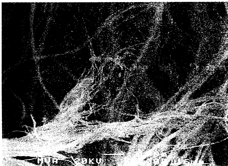
Figure 6-14. Close-up view of the surface of the gasket material shown in Figure 6-7 showing uncoated chrysotile asbestos fibers protruding.
