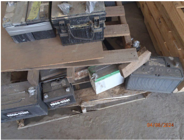
Picture 13 – Dry Dock 5 Pier F 90-Day CAA spent lead acid batteries
