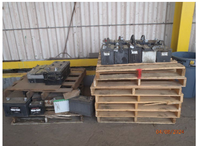
Picture 12 – Dry Dock 5 Pier F 90-Day CAA spent lead acid batteries
