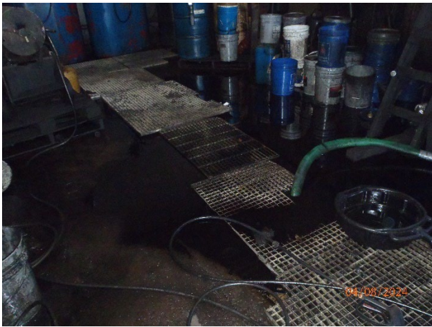
Picture 64 – Building 177 Maintenance Department used oil release to ground
