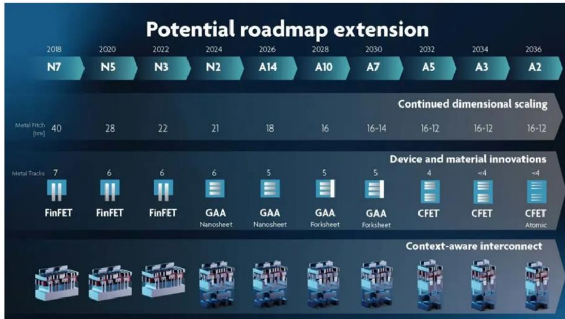
Figure B-4: IMEC’s vision of the future logic roadmap, with dimensional scaling predicted to continue through 2036 (IMEC 2023).
