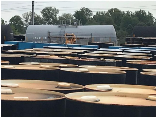
Photo 37: Bulging/Rusting containers on Permitted Pad 65.
