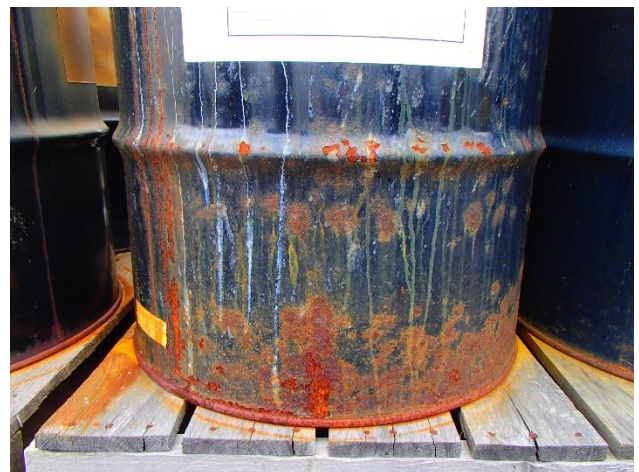
Photo 41: Bulging/Rusting containers on Permitted Pad 65.
