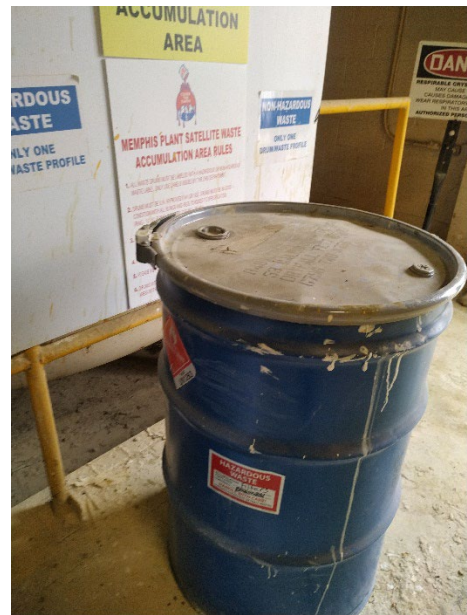
Photo 12: 55-gallon SAA container of hazardous waste in the mixing area.
