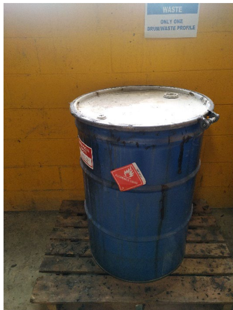
Photo 11: 55-gallon Hazardous waste SAA container near Coal Tar Line that was missing a hazardous waste label. Corrected onsite.
