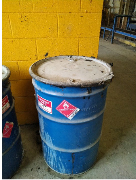
Photo 10: 55-gallon Hazardous waste SAA container near Coal Tar Line.
