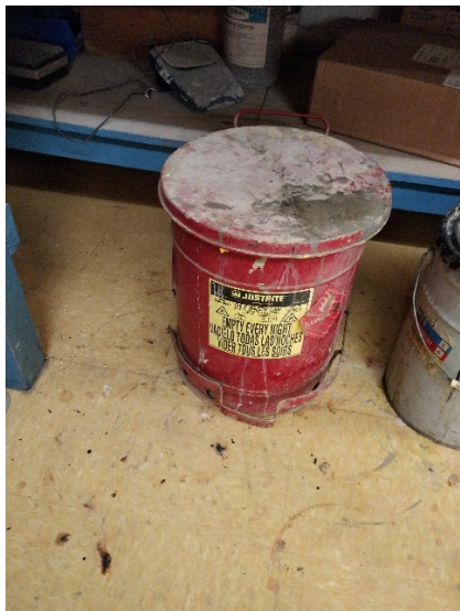
Photo 1: 5-gallon red container used to store solvent-contaminated wipes missing a hazardous waste label on it in the QC Laboratory.
