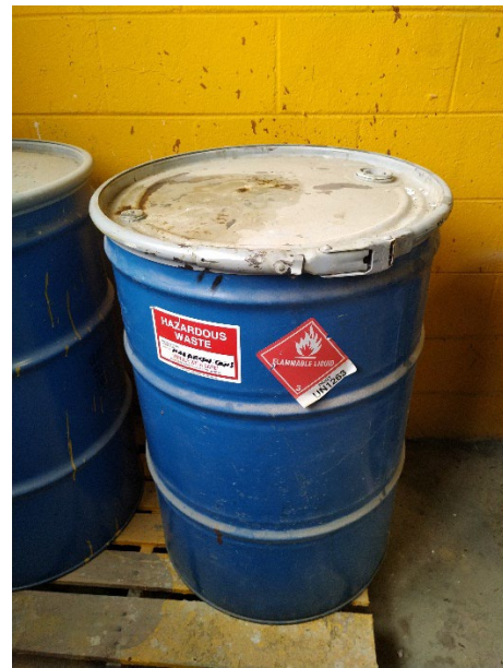
Photo 8: 55-gallon Hazardous waste SAA container near Coal Tar Line.
