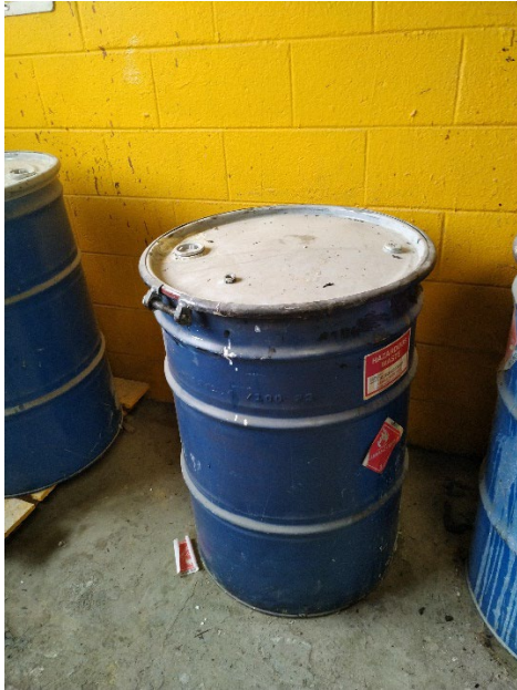
Photo 9: 55-gallon Hazardous waste SAA container near Coal Tar Line.
