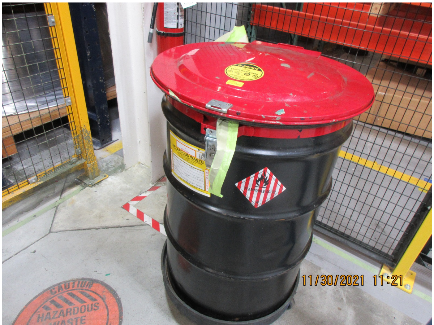
Photo 13 – Container of paint waste solids outside of procoat paint booth.
