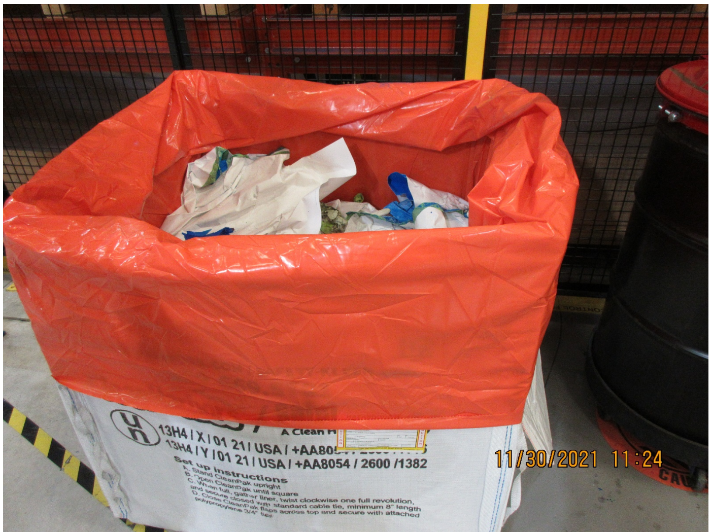
Photo 15 – Container of paint waste solids outside of procoat paint booth.
