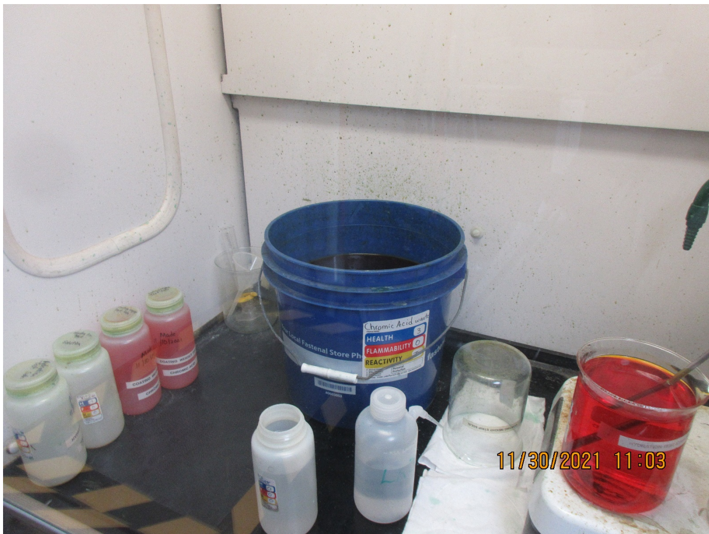
Photo 7 – Chromic acid hazardous waste in blue container in QC lab hood.
