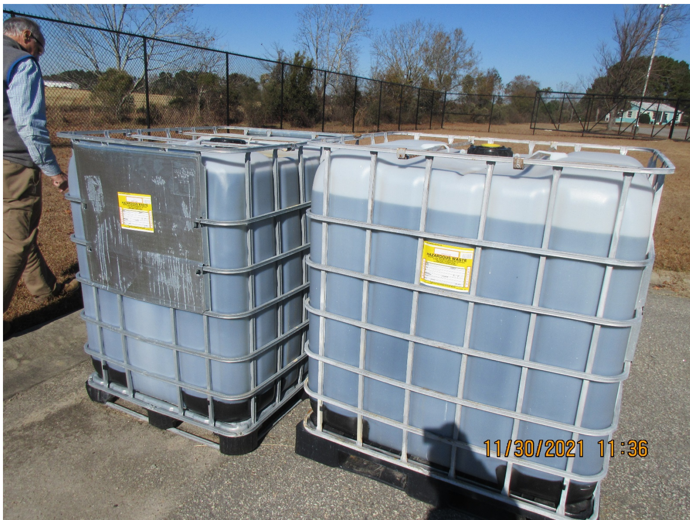
Photo 19 – Two totes of waste acid from the facility’s anodizing line on a pad in the area outside of the facility’s 90-day Hazardous Waste Accumulation Building
