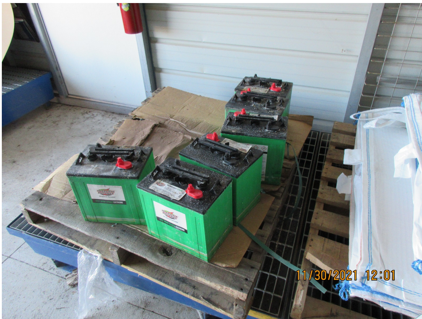
Photo 31 – Universal Waste Batteries in 90-day accumulation area
