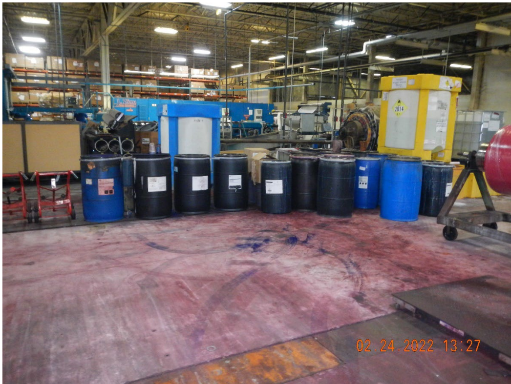
Figure 10. Drums of Powdered Dyes Stored in Production Area and Residuals
