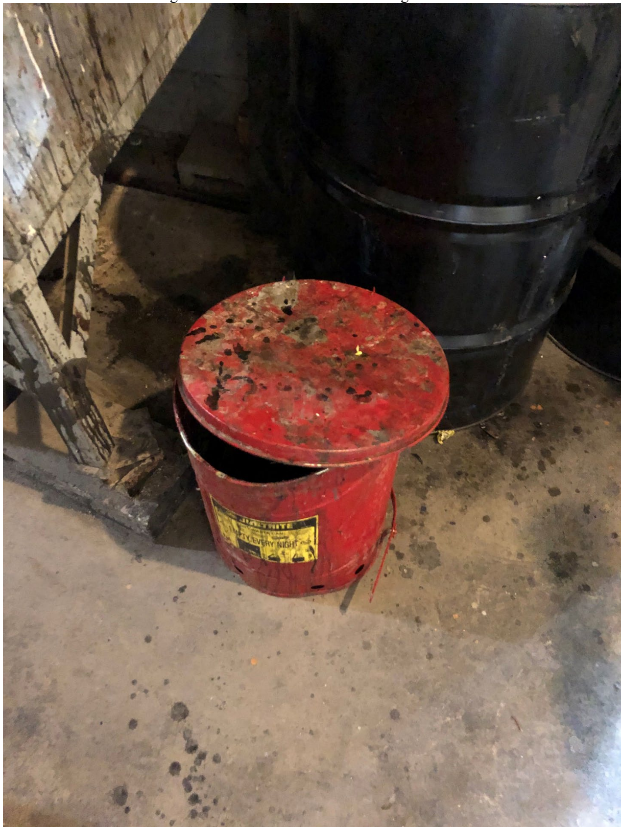
Photo #1: View of the 5-gallon metal container where used rags are stored.
