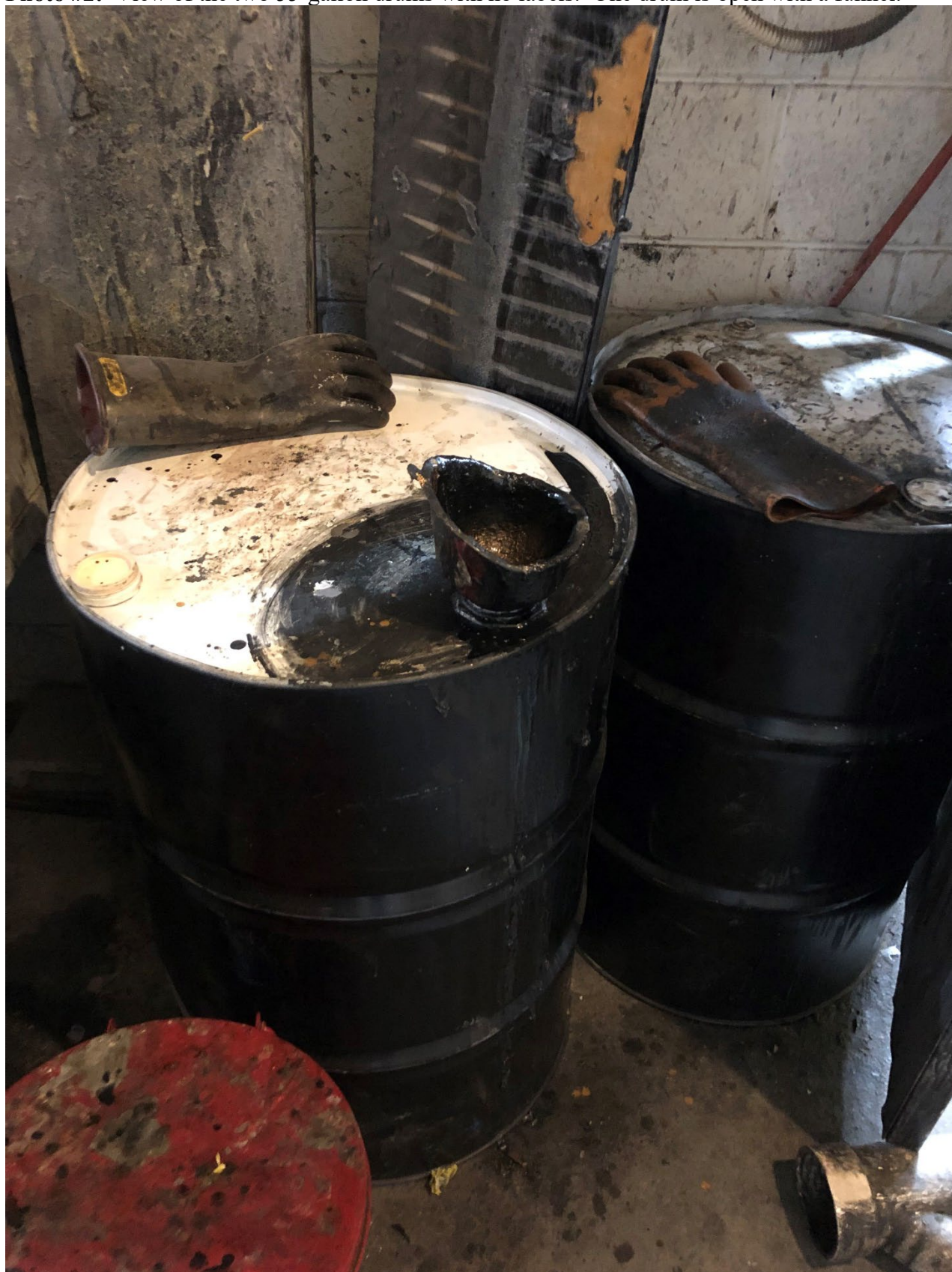
Photo #2: View of the two 55-gallon drums with no labels. One drum is open with a funnel.
